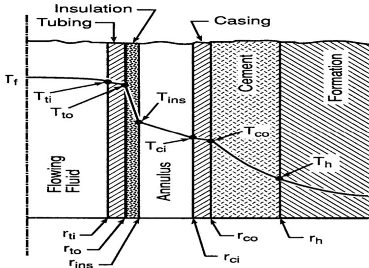
**Figure 1:** Schematic diagram of Producing and Injection Gas Well
