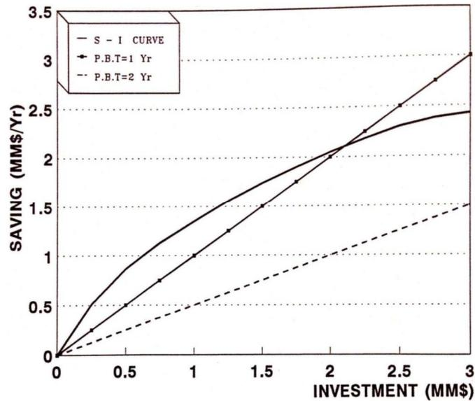
**Figure 13:** Figure for S-I for the refinery exchangers, [9]
