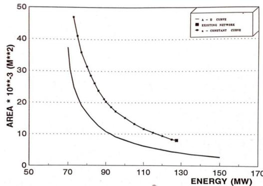
**Figure 11:** Figure of  $\alpha$ -constant with the curve of A-E for the network of Isfahan refinery
