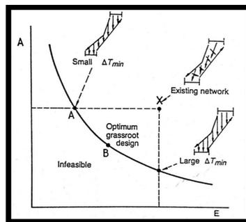
**Figure 4:** Minimum value of energy usage and the temperature, the area (A) and energy (E), [4]
