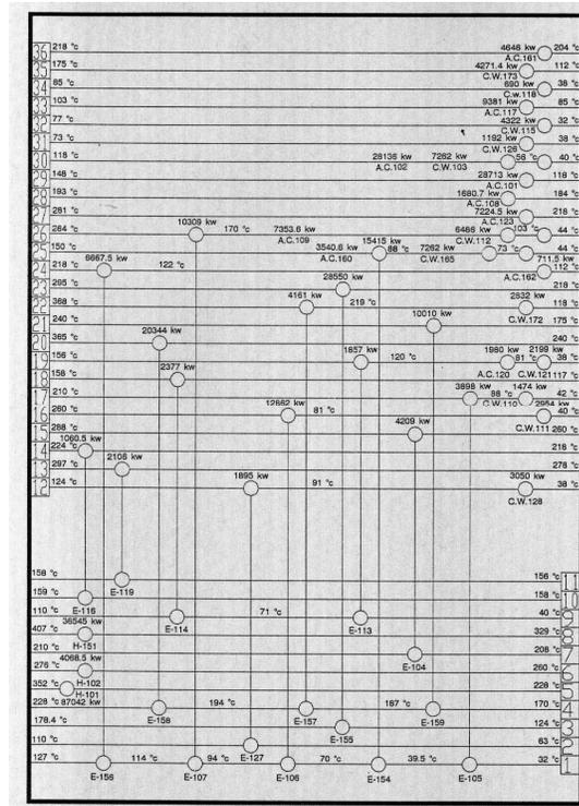
**Figure 9:** Exchanger view window for the capacity of 150,000, Isfahan refinery
