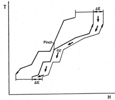
Figure 6: The passing temperature ( $\Delta E$ ) from pinch point, [7]
