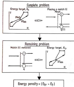
**Figure 7:** The remaining energy with fixed  $\Delta T_{min}$ , [7]
