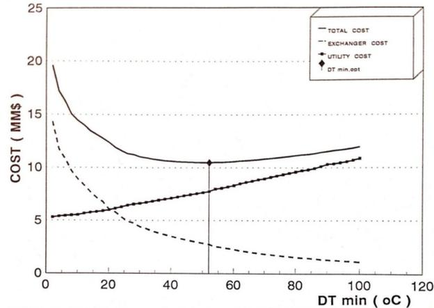
**Figure 14:** network refinery,  $\Delta T_{\min, \text{opt}}$  [14]
