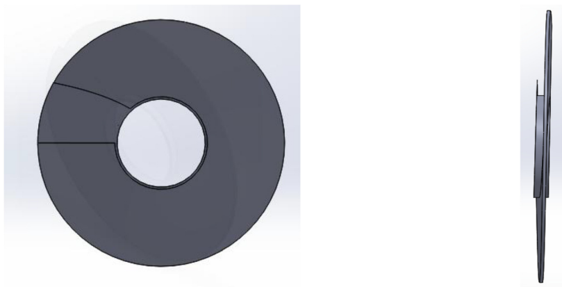
Figure 2: Front and side view section of the finned tube
