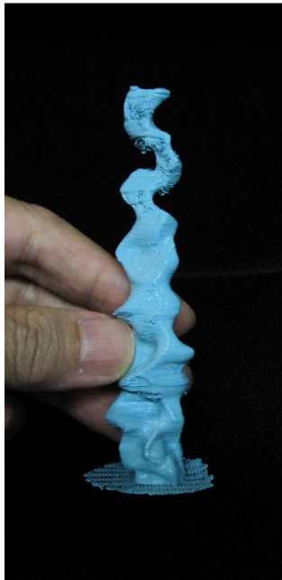
Figure 12: 3D model of flame front ( U_{A1} = 10 m/s) using a 3D printer
