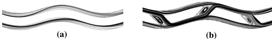
Figure 19: The streamlines in x-y plane (x(4-6)mm) & elevation-z=0.3mm)-Re(600) in (a) WWOC and (b) WAOC
