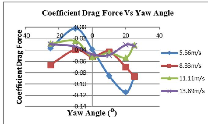
**Figure 17:** Coefficient of Drag Force at different Yaw Angles with 4 different speeds.
