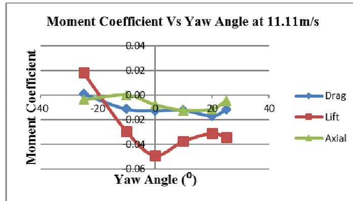
**Figure 15:** Moment Coefficient at different Yaw Angle at 11.11m/s.
