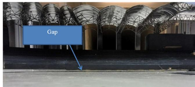
**Figure 6:** Gap between the Model and the Floor Surface.
