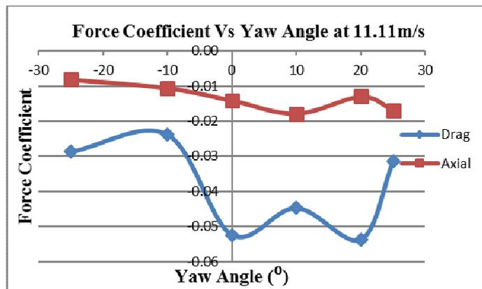
**Figure 11:** Force Coefficient at different Yaw Angle at 11.11m/s
