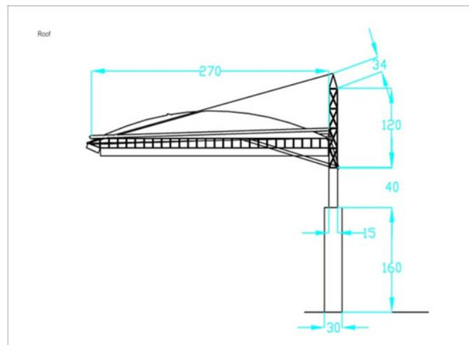
**Figure 5(b):** Side view and dimensions of the UTM sport complex.
