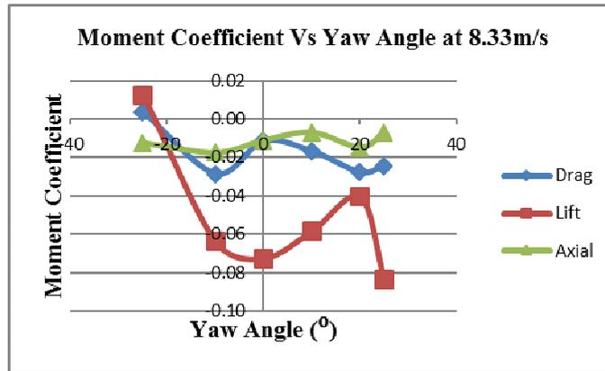
**Figure 14:** Moment Coefficient at different Yaw Angle at 8.33m/s
