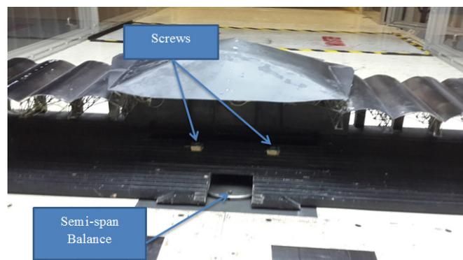
**Figure 7:** Attachment model to the Semi-Span Balance.
