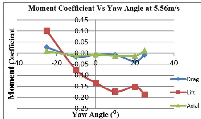
**Figure 13:** Moment Coefficient at different Yaw Angle at 5.56m/s.
