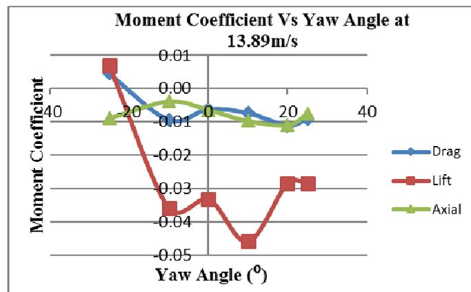
**Figure 16:** Moment Coefficient at different Yaw Angle at 13.89m/s
