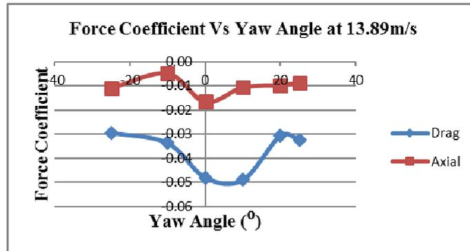
**Figure 12:** Force Coefficient at different Yaw Angle at 13.89m/s
