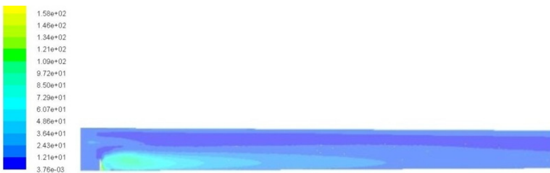
Fig. 11. Turbulent intensities contour on vertical plane bisecting turbine hub
