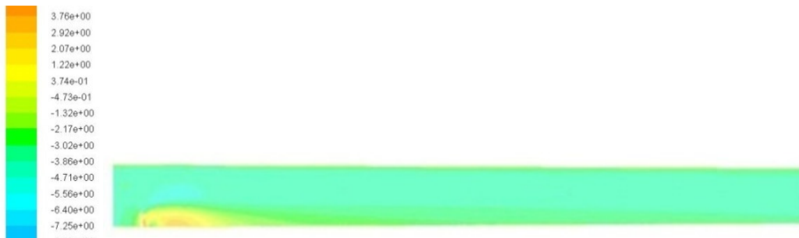
Fig. 10. Streamline velocity contour on vertical plane bisecting turbine hub
