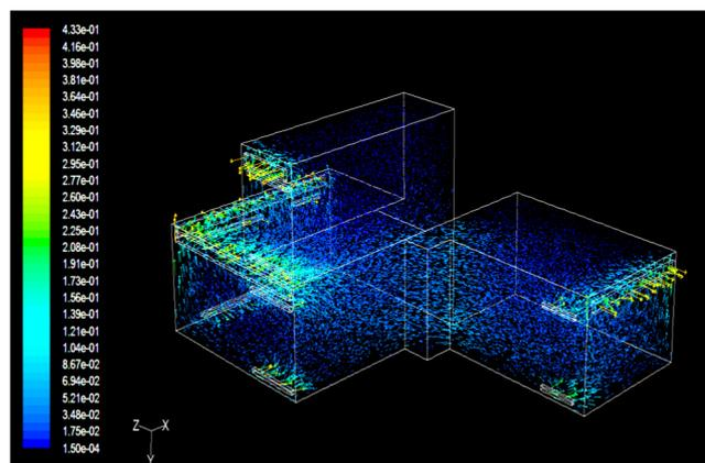
**Fig. 5.** Air-flow distribution (m/s) inside the house when gable vents are used
