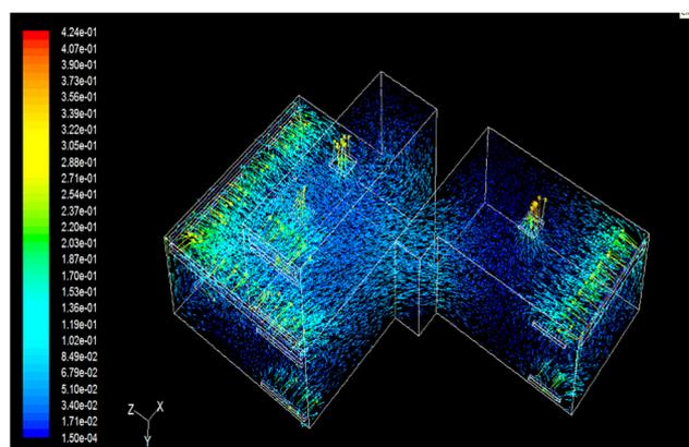
**Fig. 6.** Air-flow distribution (m/s) inside the house when a combination of solar chimneys and gable vents are used
