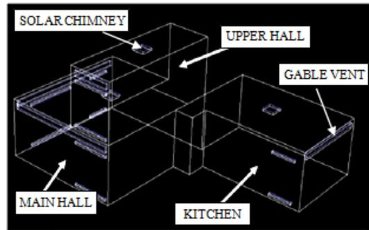
**Fig. 1.** A representative model of the house considered for the CFD computational domain (rear view)
