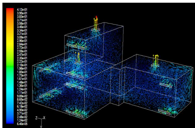
**Fig. 4.** Air-flow distribution (m/s) inside the house when solar chimney ventilation is used
