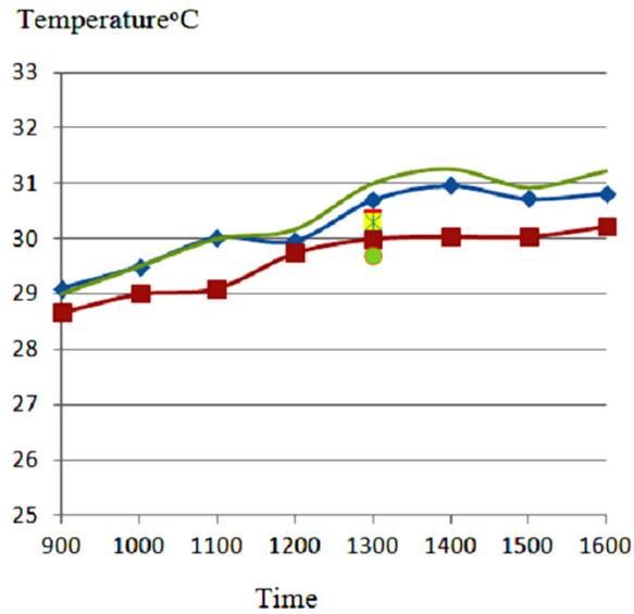
**Fig. 2.** Comparison between the average air temperatures obtained from the CFD simulation and the measured values
