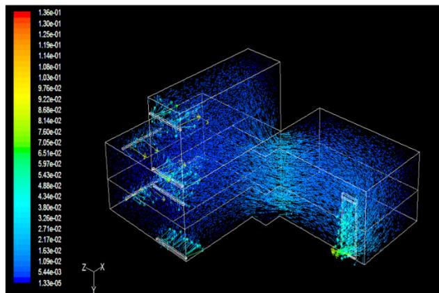
**Fig. 3.** Air-flow distribution (m/s) inside the house when the door on eastern wall of the kitchen is left opened
