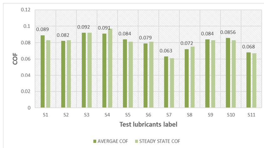
Fig. 5. COF of vegetable based and mineral lubricant
