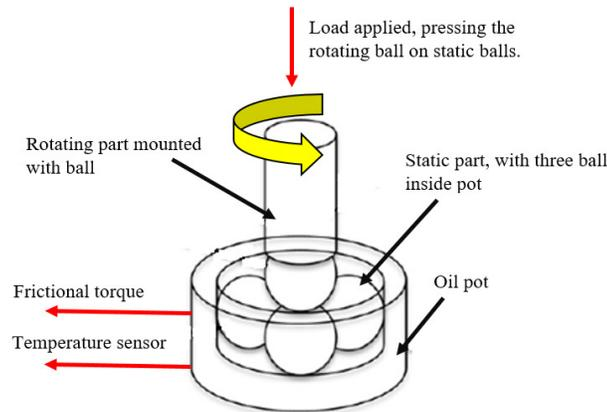
**Fig. 2.** Schematic diagram of four ball tribotester
