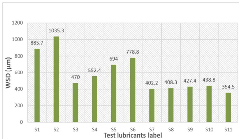
**Fig. 4.** WSD of vegetable based and mineral lubricant
