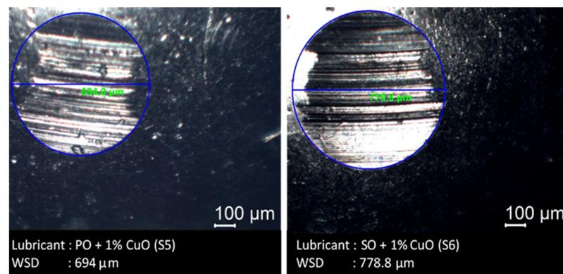
**Fig. 3(c).** WSD of S5 and S6 lubricants
