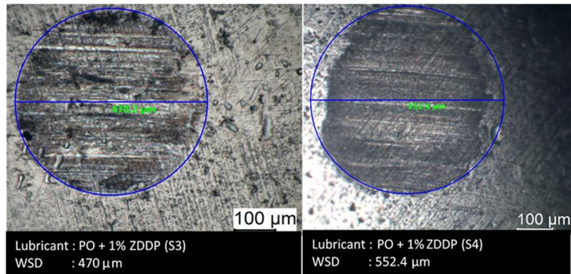
**Fig. 3(b).** WSD of S3 and S4 lubricants
