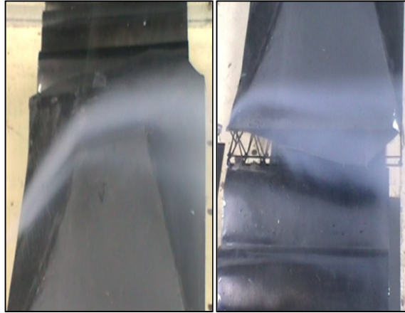
Fig. 8. Flow visualisation on top and side of the Grandstand
