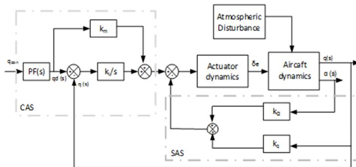
Fig. 3. Pitch rate command /attitude hold controller architecture.
