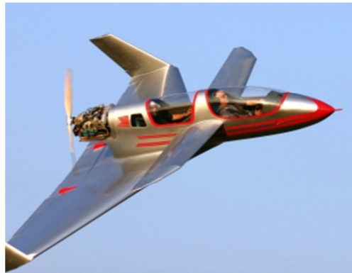
Fig. 1. The Bateliur - a surveillance and patrol aircraft that utilize the delta wing with rear propeller configuration
