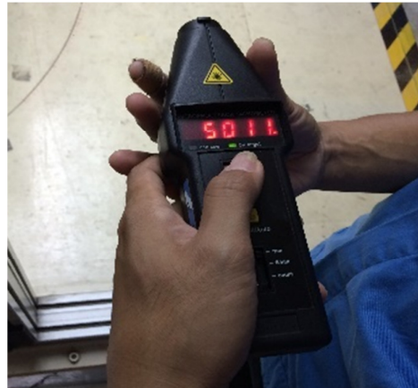
Fig. 4. Tachometer to measure the propeller speed
