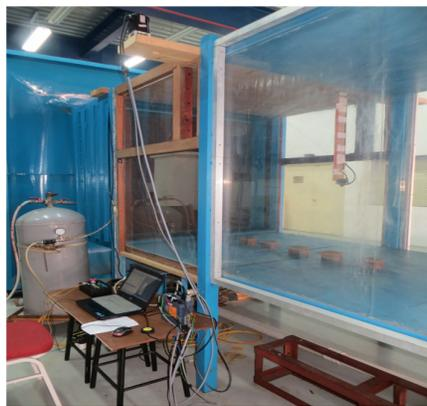
**Fig. 5.** Experimental set up for testing the spray nozzle in the wind tunnel
