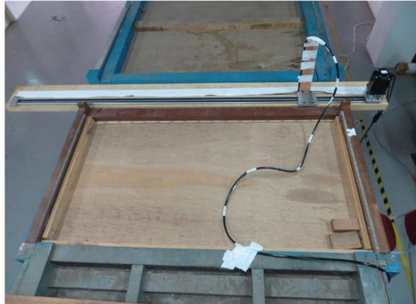
**Fig. 4.** Installation of the spray mechanism (linear motion system) above the wind tunnel
