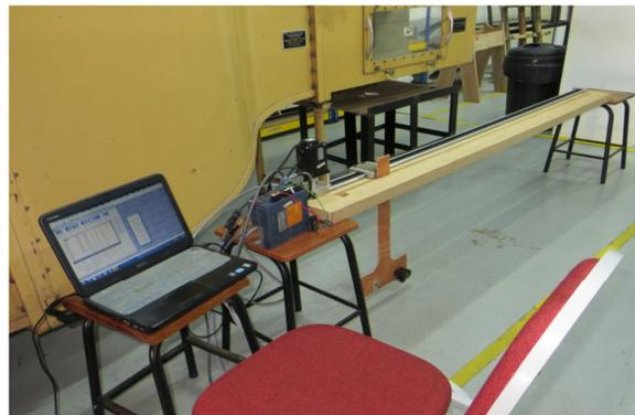
**Fig. 3.** Experimental set up for testing the speed of the linear motion system
