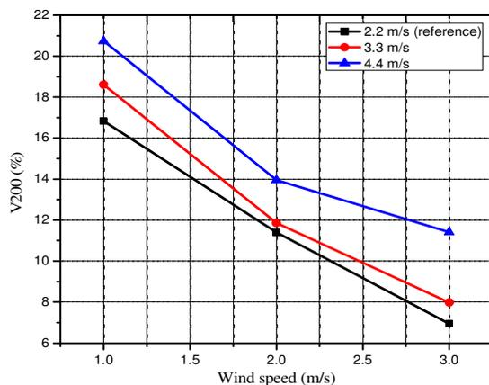
**Fig. 8.** Graph of V200 vs wind speed for the spray nozzle at three sprayer speeds
