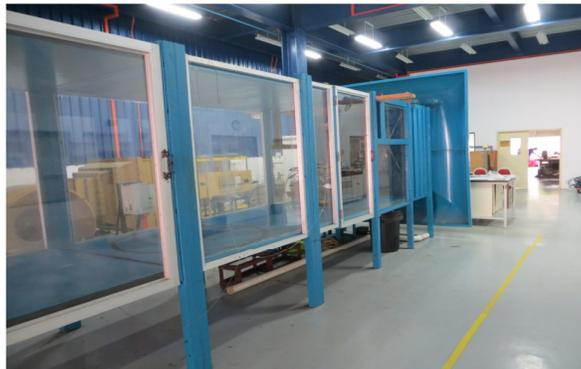
**Fig. 1.** Subsonic wind tunnel
