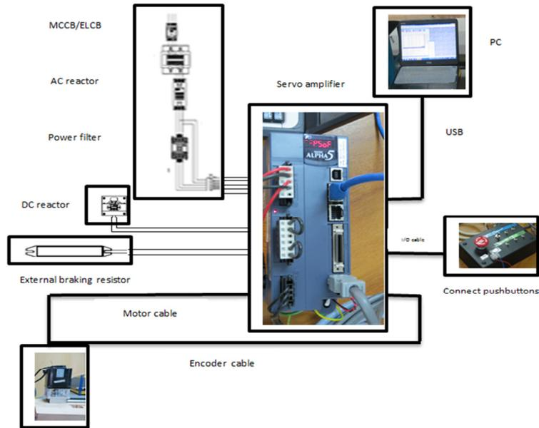
**Fig. 2.** Connecting diagram of the linear motion system
