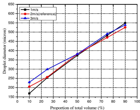
**Fig. 7.** Graph of droplet diameters vs proportion of total volume for spray nozzle at driving speed of 2.2 m/s under effect three wind speeds
