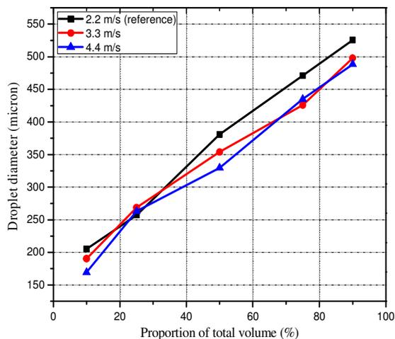
**Fig. 6.** Graph of droplet diameters vs proportion of the total volume for the spray nozzle at three sprayer speeds under effect wind speed of 2 m/s
