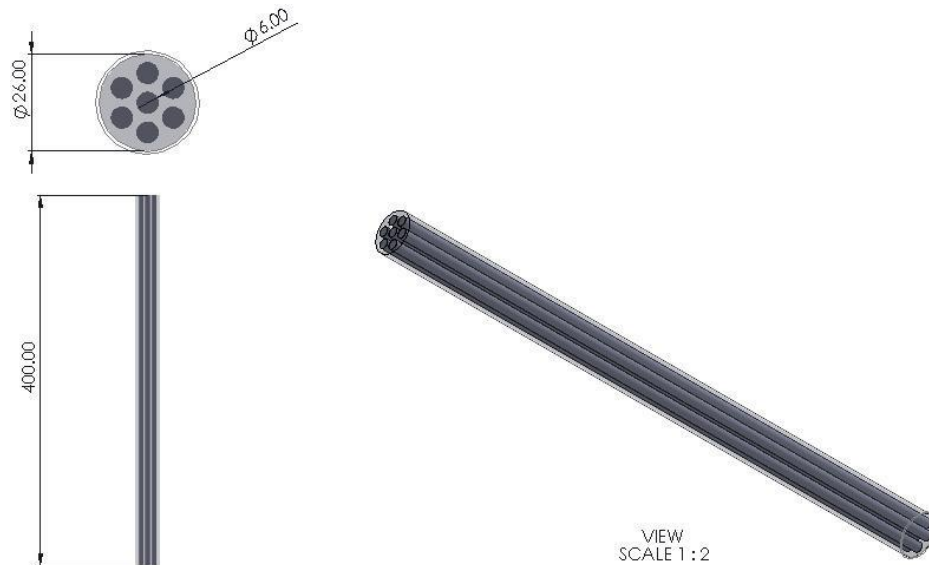
Fig. 2. Inside drawing of the membrane reactor
