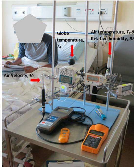
**Fig. 1.** Measurement equipment for  $T_a$ ,  $T_g$ ,  $V_a$  and  $RH$  setup on trolley
