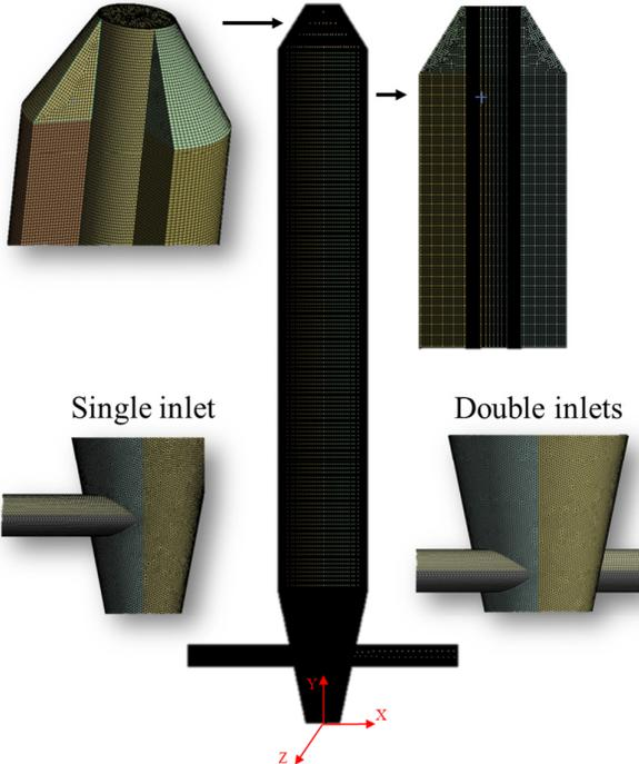
Fig. 5. Generated rectangular grid for the numerical mode
