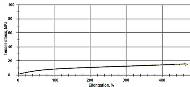
**Fig. 10.** Tensile curve at break (Without aging)
