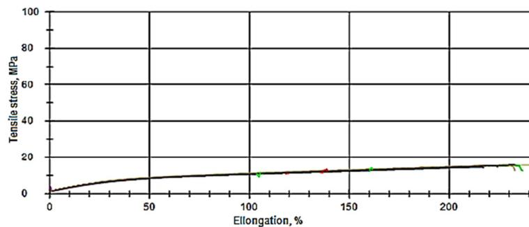
**Fig. 5.** Resistance strength versus elongation at break (without aging)
