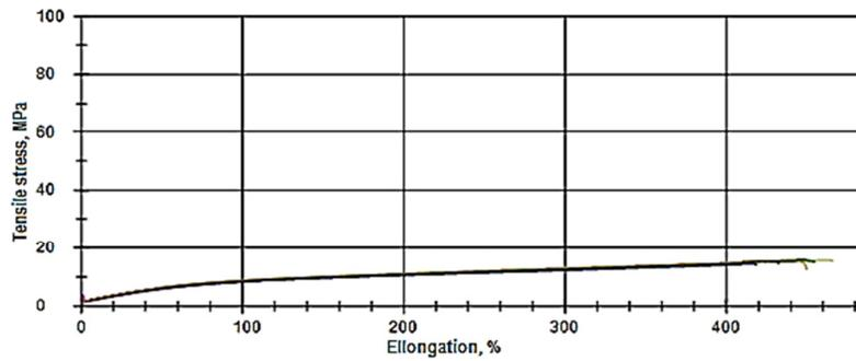
**Fig. 8.** Tensile curve at break (After aging)
