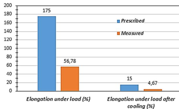
Fig. 13. Elongation test under load and hot results validated with prescribed values
