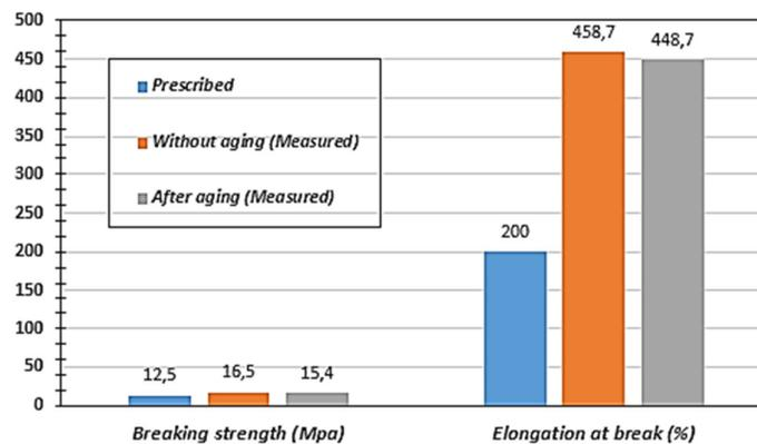
Fig. 12. Validation of results with those of IEC recommendations, (7 days @ 135 °C)
