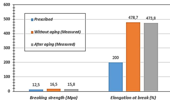
**Fig. 9.** Validation of results with those of IEC recommendations, (7 days @ 100 °C)
