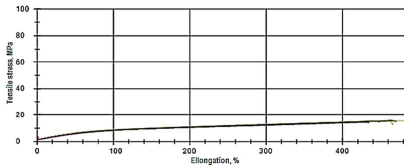
**Fig. 7.** Tensile curve at break (Without aging)
