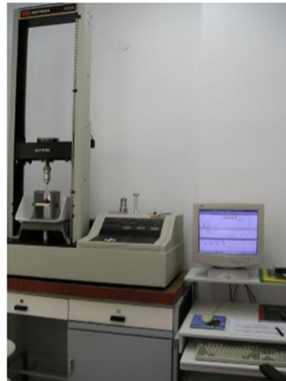
**Fig. 2.** Universal testing machine Instron4301
