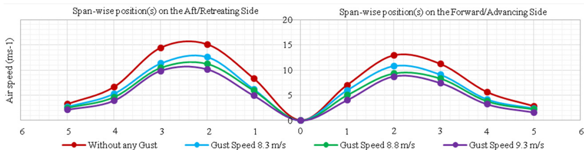
Fig. 9. Span-wise airspeed (or lift/thrust) distribution on the main rotor of the subscale helicopter for both with and without the manifestation of active gusts during forward flight
