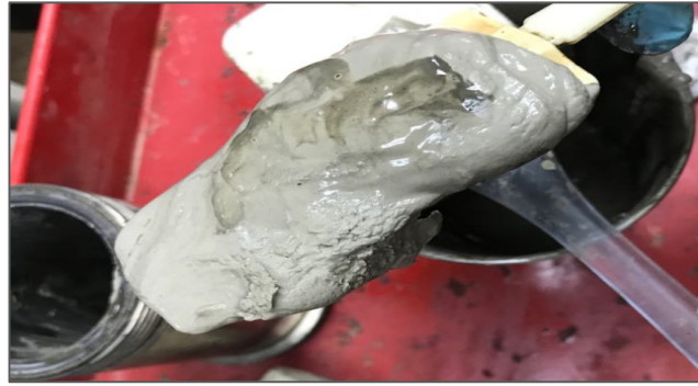
Fig. 6. Barite sagging due to low LSRV
