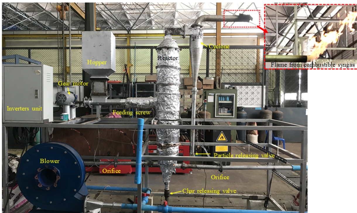
Fig. 5. The photo of mini pilot fluidized-bed gasifier system
