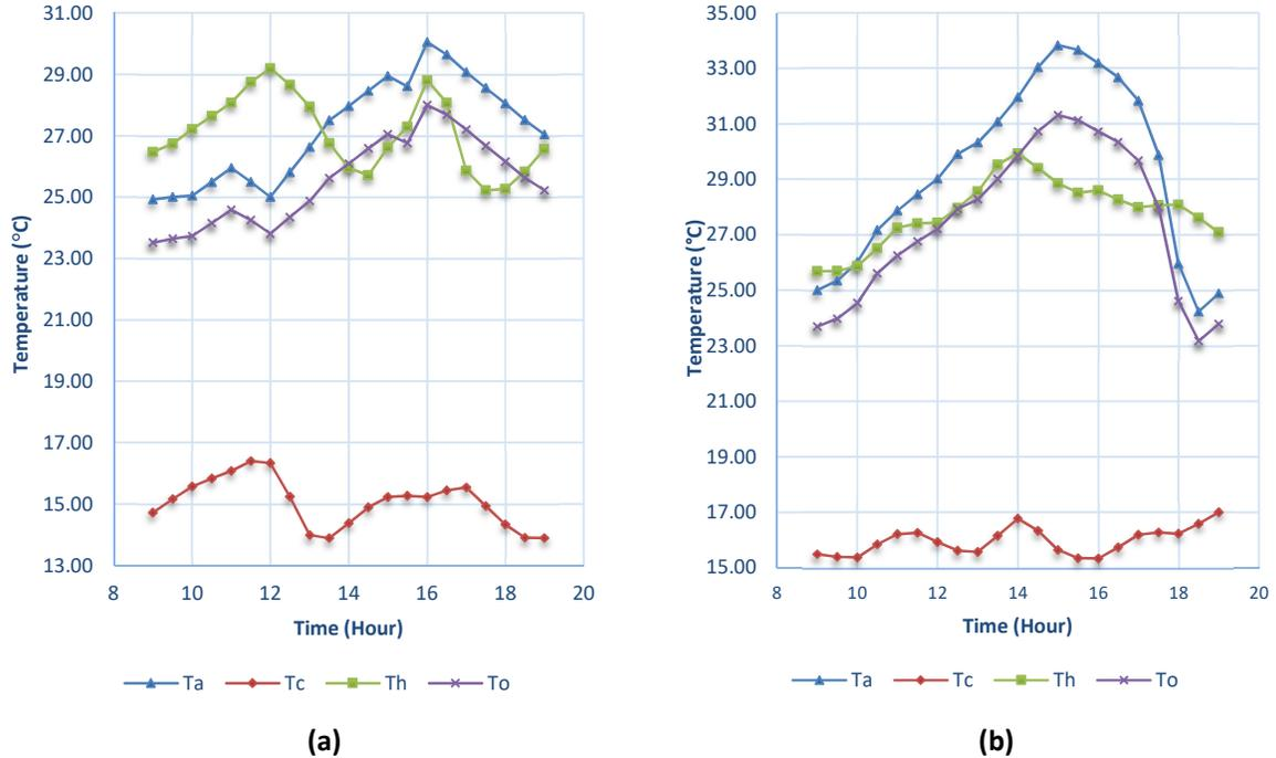
**Fig. 5.** Hourly temperature reduction of TE Cooling System in **(a)** Day 1 and **(b)** Day 2 ( $V_{air} = 0.10$  m/s;  $I = 6$  A).
