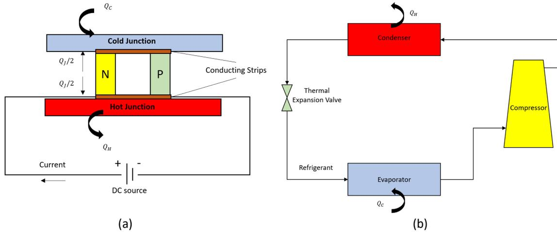
**Fig. 1.** Schematic drawing of **(a)** TEM cooling process with **(b)** refrigeration cycle
