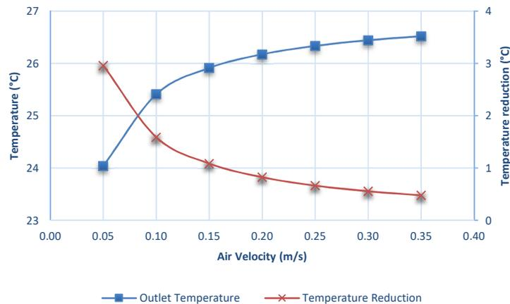
**Fig. 6.** Variation of outlet temperature with different inlet air velocity ( $T_a = 27^\circ\text{C}$ ;  $I = 6$  A)
