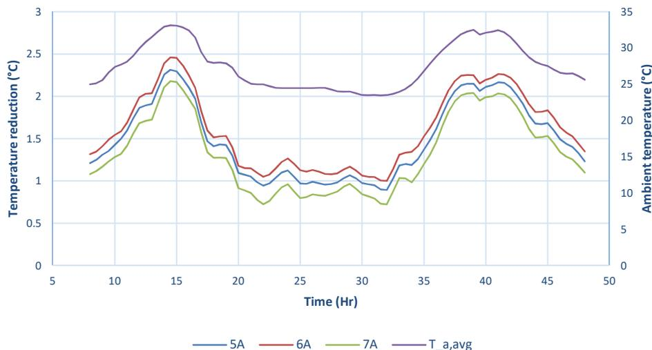
**Fig. 4.** Hourly temperature reduction of TE cooling system at various operating currents ( $V_{air} = 0.1$  m/s).
