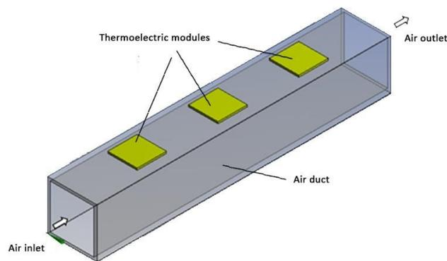
**Fig. 2.** Configuration of TE Cooling System.
