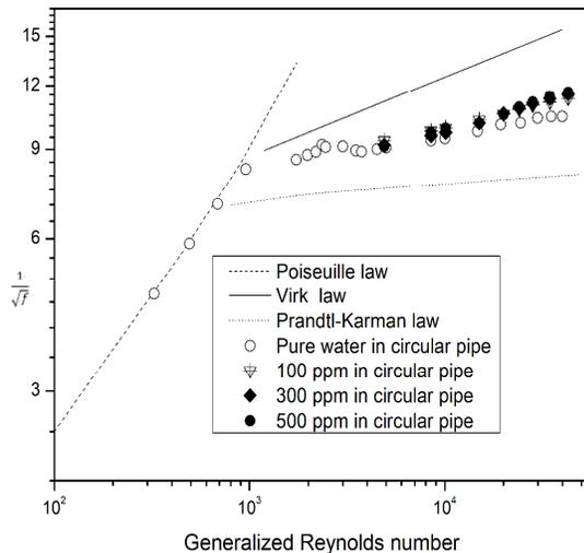
**Fig. 5.** Comparison of generalized Reynolds number versus the friction factor in a circular pipe
