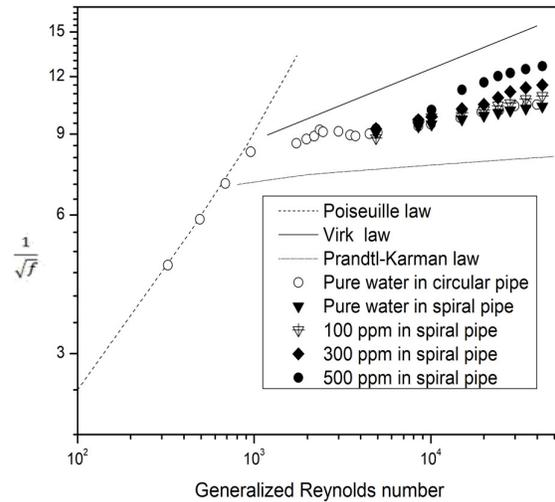
**Fig 6.** Comparison of generalized Reynolds number versus the friction factor in a spiral pipe
