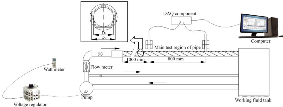
**Fig. 1.** Experimental set-up
