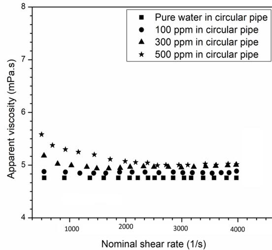
**Fig. 4.** Apparent viscosity of CaCO<sub>3</sub> solution in a circular pipe
