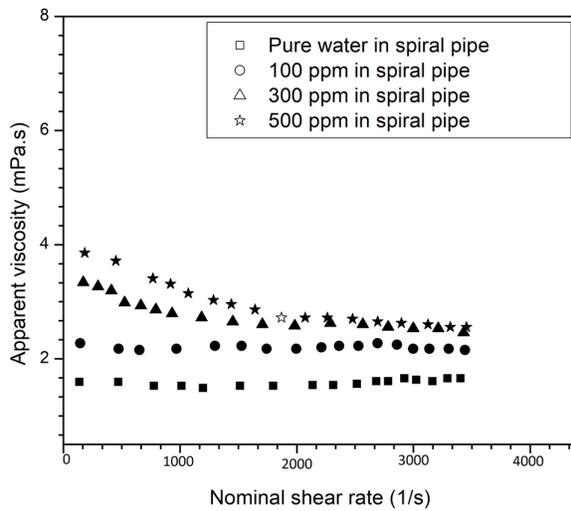
**Fig. 3.** Apparent viscosity of CaCO<sub>3</sub> in a spiral pipe
