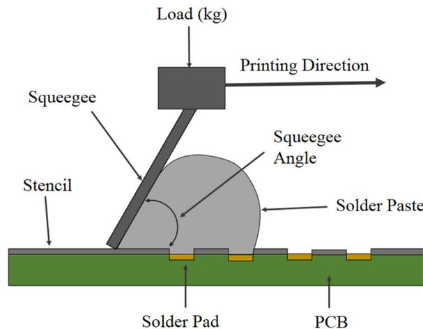
Fig. 1. Solder Paste Stencil Printing Process
