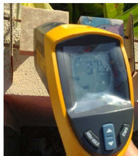
Fig. 8. The temperature of the top surface of specimen is measured and recorded
