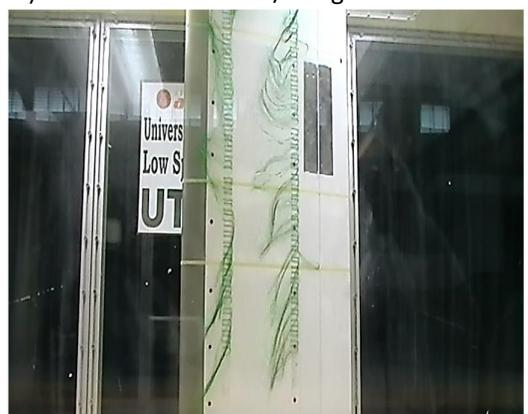
f) Reversed flow condition during tuft testing
