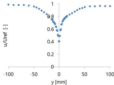
**Fig. 4.** Velocity profile at  $x=10\text{mm}$  downstream the airfoil
