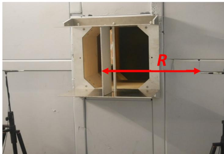
**Fig. 5.** Microphones position for sound measurement
