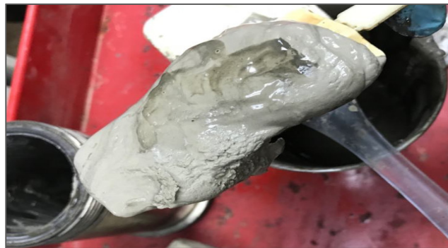
Fig. 6. Barite sagging due to low LSRV
