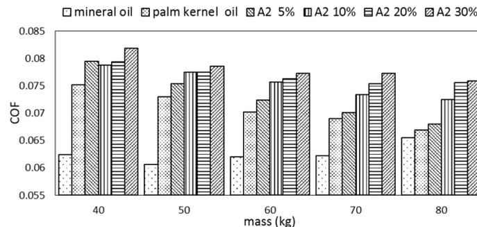
Fig. 4. Coefficient of friction against load
