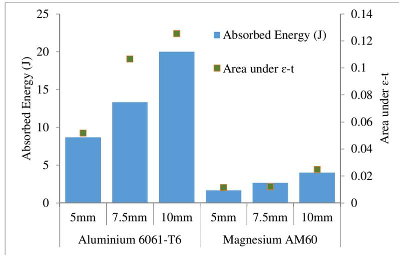
**Fig. 16.** Correlation of Absorbed Energy and Area under Strain-Time Graph at Speed of 5.18m/s
