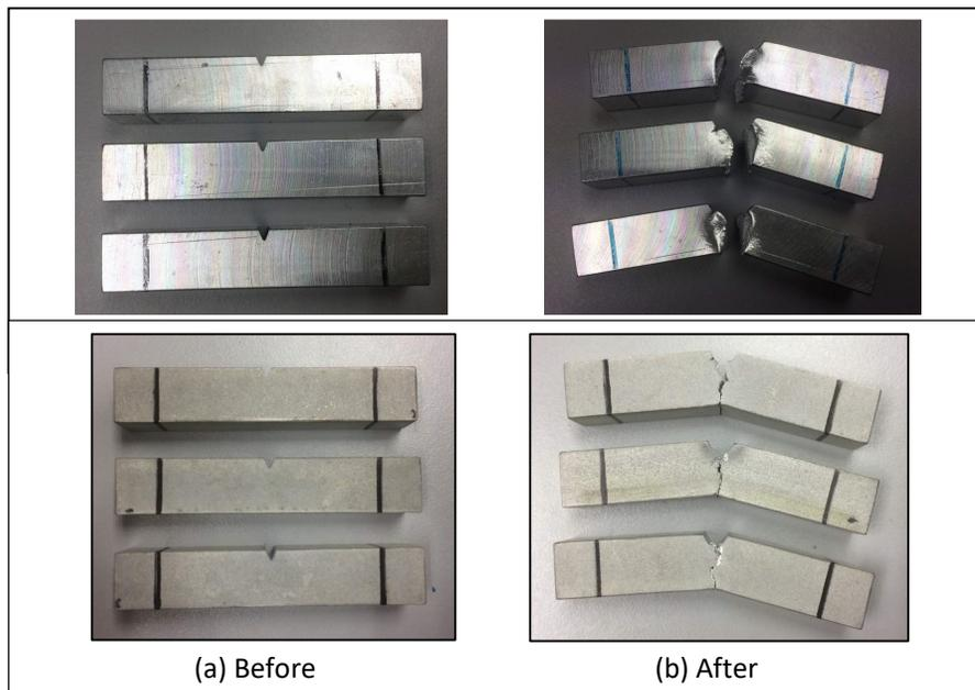
**Fig. 4.** Specimens of Magnesium AM60 before and after impact test
