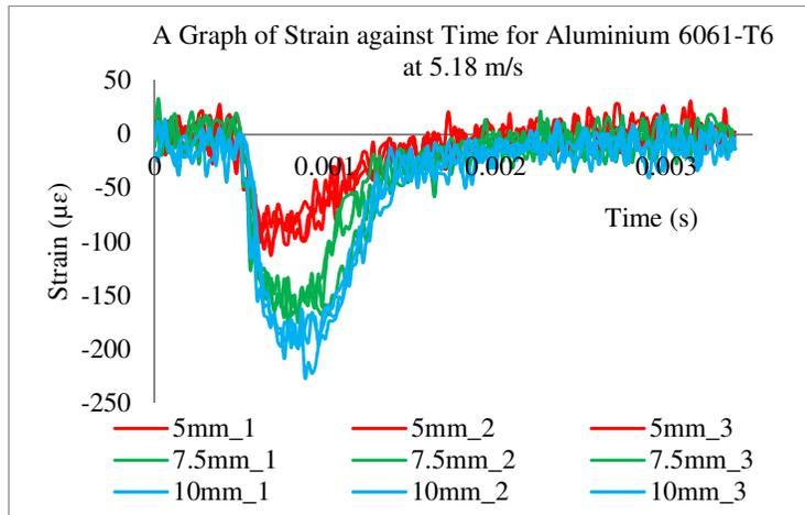
**Fig. 10.** A Graph of Strain-Time Graph of Aluminium 6061-T6 at 5.18 m/s for Different Thickness
