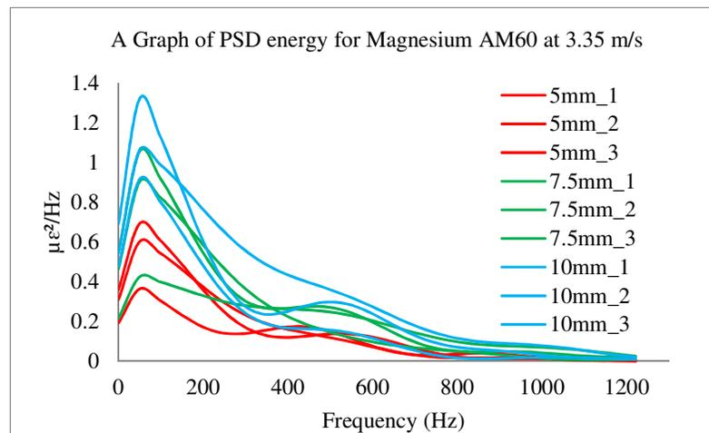
**Fig. 7.** PSD Energy Graph for Magnesium AM60 at Impact Speed of 3.35 m/s for Different Thicknesses
