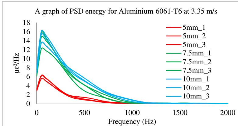
**Fig. 5.** PSD Energy Graph for Aluminium 6061-T6 at Impact Speed of 3.35 m/s for Different Thicknesses
