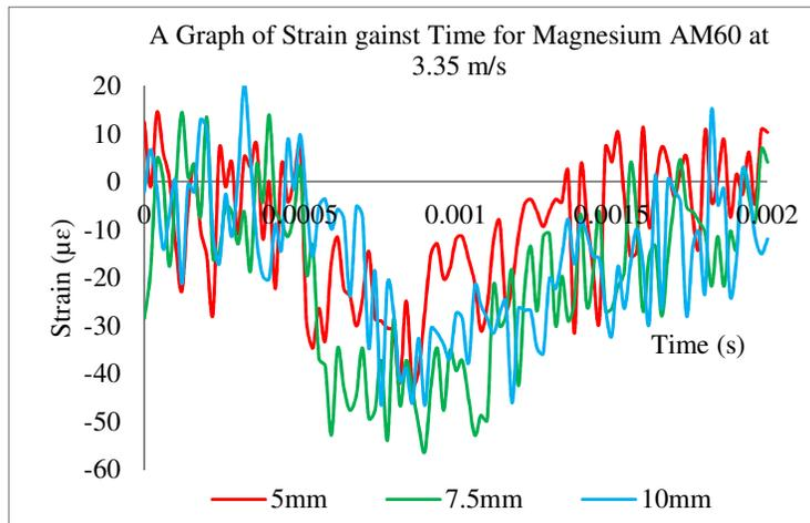
**Fig. 11.** A Graph of Strain-Time Graph of Magnesium AM60 at 3.35 m/s for Different Thickness
