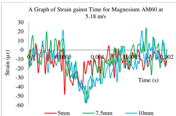
**Fig. 12.** A Graph of Strain-Time Graph of Magnesium AM60 at 5.18 m/s for Different Thickness
