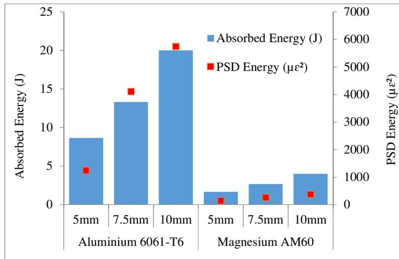
**Fig. 14.** Correlation of Absorbed Energy and PSD Energy at Speed of 5.18 m/s
