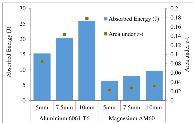
**Fig. 15.** Correlation of Absorbed Energy and Area under Strain-Time Graph at Speed of 3.35 m/s
