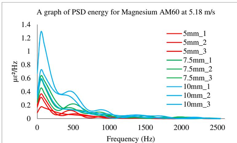
**Fig. 8.** PSD Energy Graph for Magnesium AM60 at Impact Speed of 5.18 m/s for Different Thicknesses
