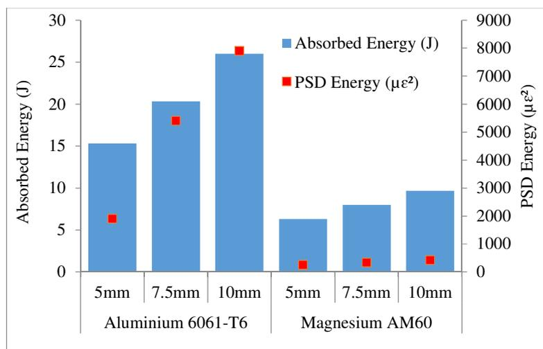
**Fig. 13.** Correlation of Absorbed Energy and PSD Energy at Speed of 3.35 m/s
