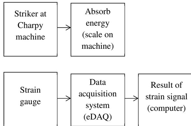
Fig. 3. Apparatus connection for data collection
