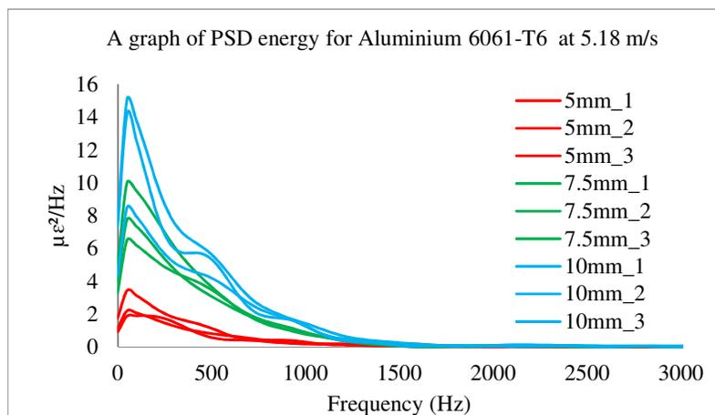
**Fig. 6.** PSD Energy Graph for Aluminium 6061-T6 at Impact Speed of 5.18 m/s for Different Thicknesses
