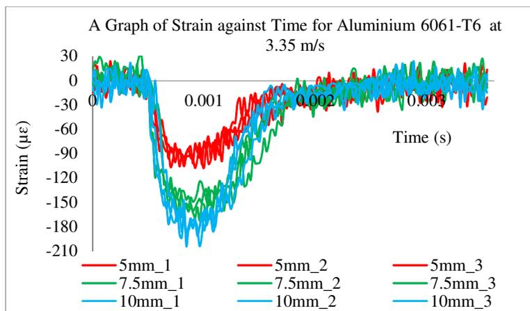
**Fig. 9.** A Graph of Strain-Time Graph of Aluminium 6061-T6 at 3.35 m/s for Different Thickness
