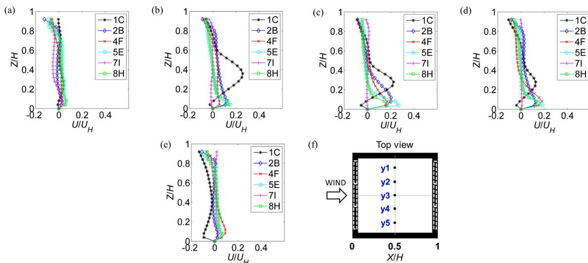
**Fig. 10.** Spanwise flow distribution inside building for cases with aligned cross openings: (a) location  $y_1$ ; (b) location  $y_2$ ; (c) location  $y_3$ ; (d) location  $y_4$ ; (e) location  $y_5$ ; (f) sampling locations
