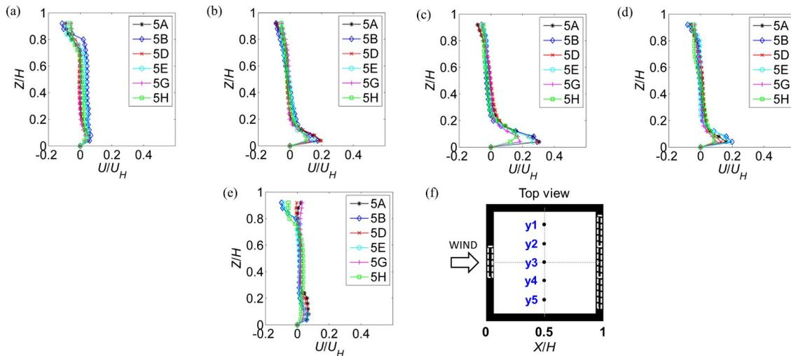
**Fig. 13.** Spanwise flow distribution inside a building for cases with different outlet positions: (a) location  $y_1$ ; (b) location  $y_2$ ; (c) location  $y_3$ ; (d) location  $y_4$ ; (e) location  $y_5$ ; (f) sampling locations
