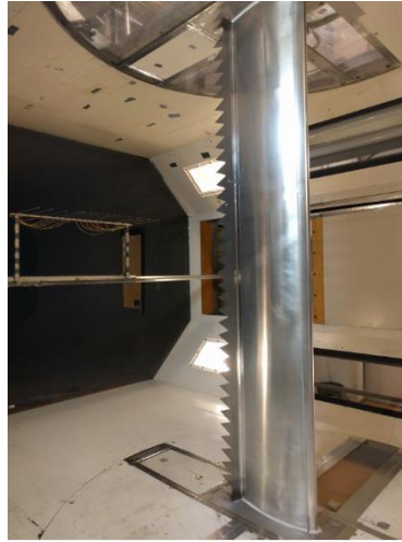
Fig. 5. Wind tunnel test model of NACA 643418 airfoil
