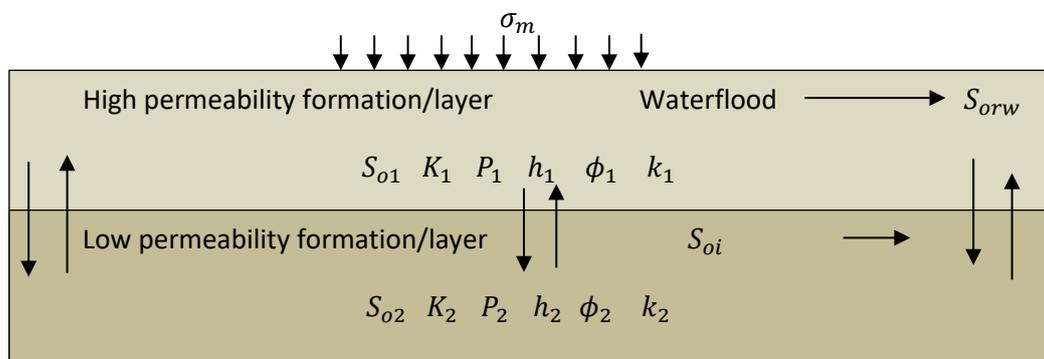
**Fig. 1.** Illustrates the two-layer oil reservoir model stimulated by the mean normal seismic stress ( $\sigma_m$ ) [51]
