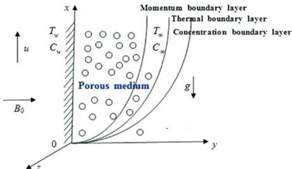
Fig. 1. The flow configuration of the problem
