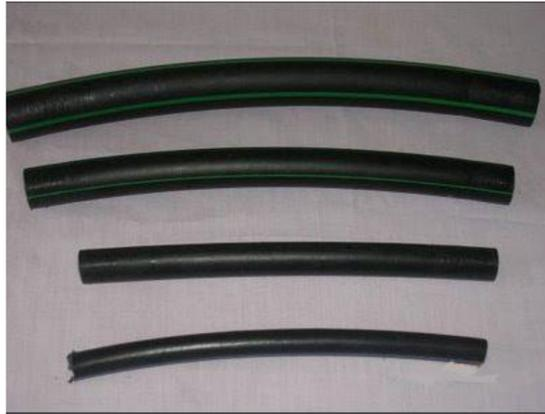
**Fig. 3.** Pipe of HDPE Material Grade PE 80 [17]
