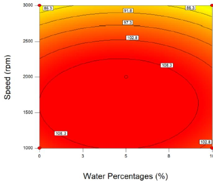
**Fig. 3.** Interactive contour plot for engine torque at difference percentages of water and speed
