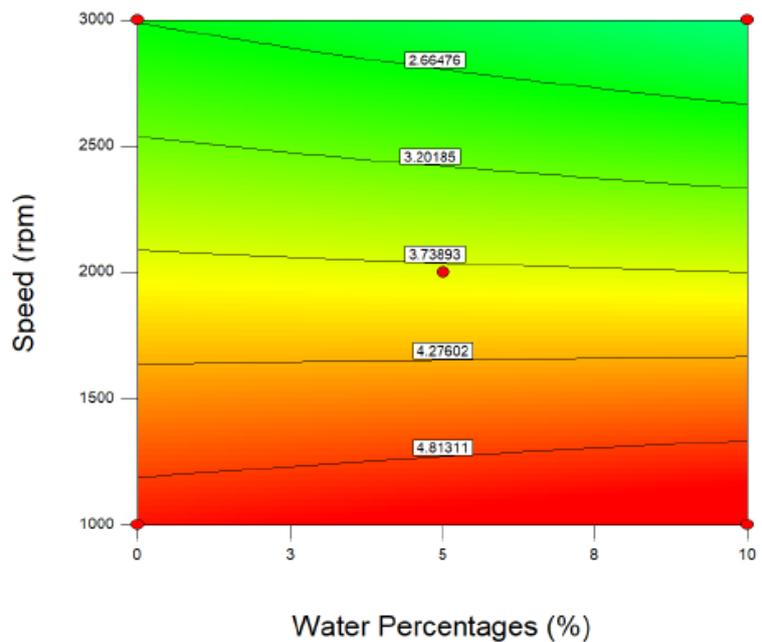
**Fig. 7.** Interactive contour plot for CO at difference percentages of water and speed
