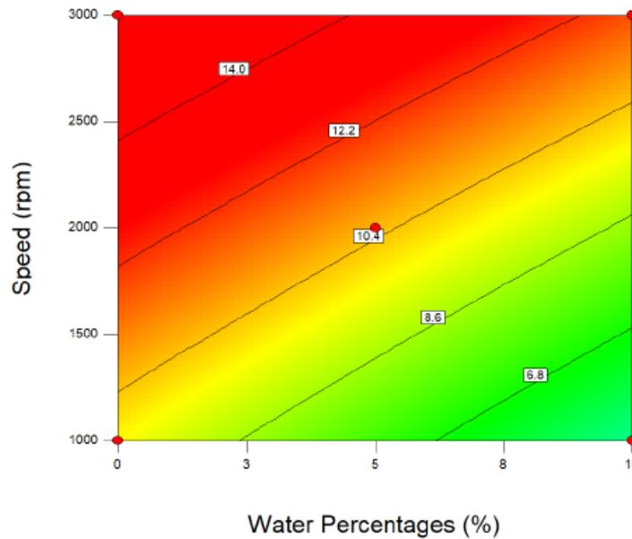
**Fig. 8.** Interactive contour plot for CO<sub>2</sub> at difference percentages of water and speed
