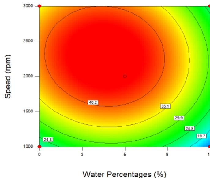
**Fig. 4.** Interactive contour plot for BTE at difference percentages of water and speed
