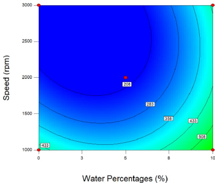
**Fig. 5.** Interactive contour plot for BSFC at difference percentages of water and speed
