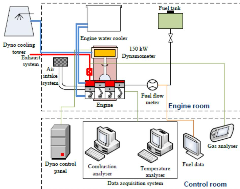
Fig. 2. Schematic diagram of the engine test rig
