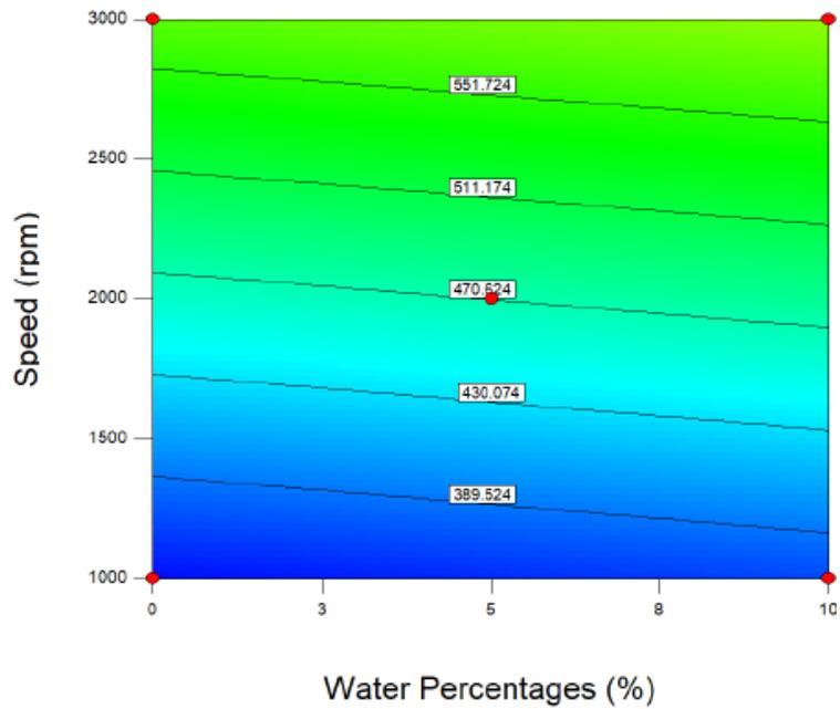
**Fig. 6.** Interactive contour plot for NOx at difference percentages of water and speed
