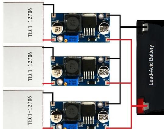
**Fig. 5.** Diagram shows the electrical connections of the TEG system
