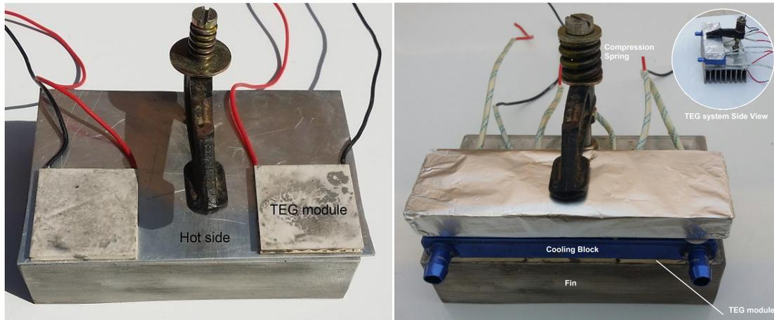
**Fig. 3.** Mechanical clamping of the TEG modules.
