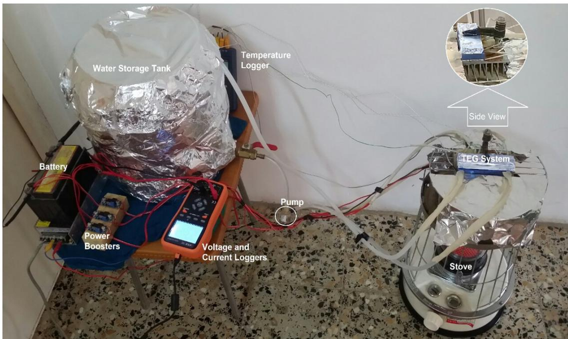
**Fig. 4.** Picture for the built TEG- stove system
