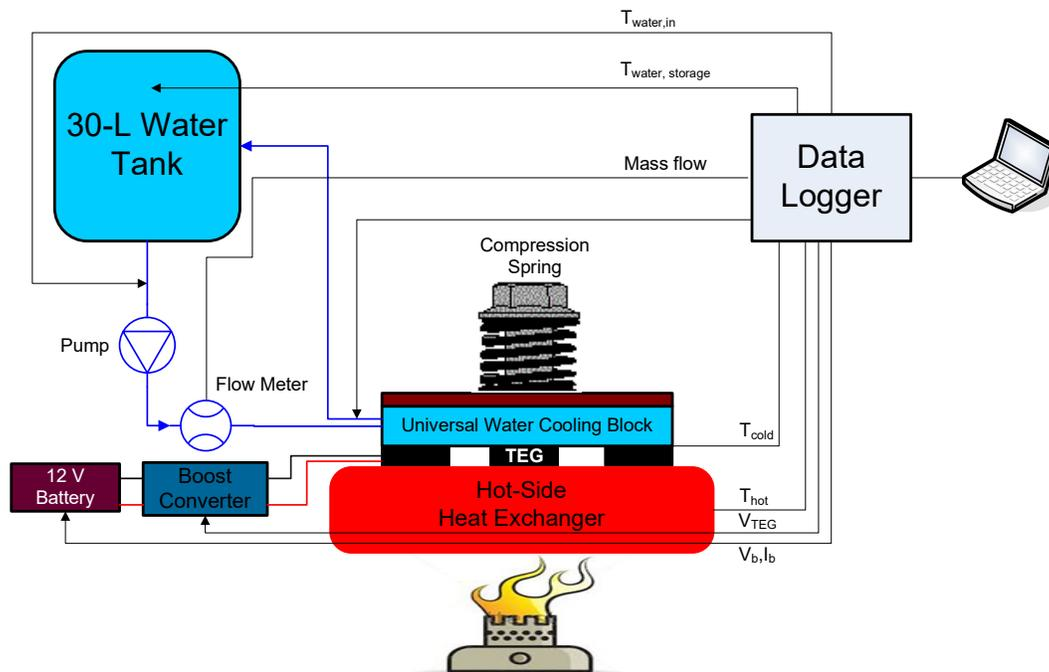
Fig. 2. Schematic of the detailing of TEG system.
