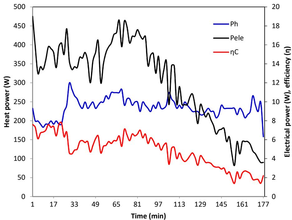
Fig. 8. Variation of thermal power ( $P_h$ ), output power ( $P_{ele}$ ) and TEG efficiency ( $\eta$ ) versus time of the experiment
