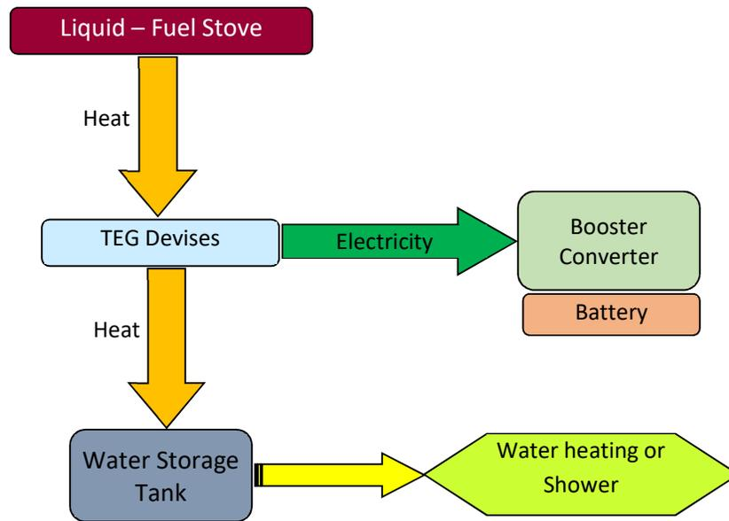
Fig. 1. Energy diagram of the built TEG system
