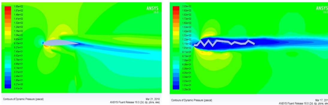
**Fig. 22.** Dynamic Pressure and Velocity Magnitude contours at AOA= 10 Deg, V= 11.8 m/s
