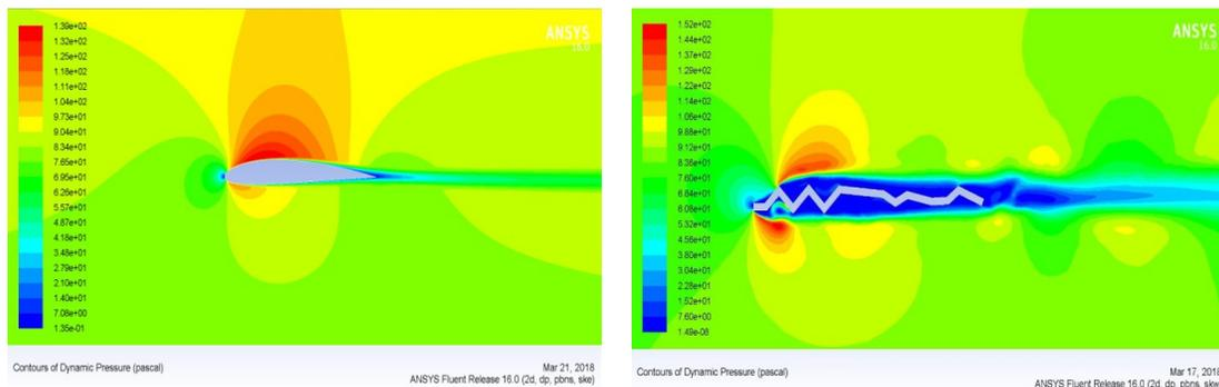
**Fig. 21.** Dynamic Pressure and Velocity Magnitude contours at AOA= 5 Deg,  $V = 11.8$  m/s
