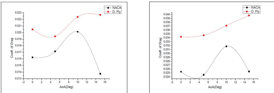
Fig. 17.  $C_d$  vs AoA plot for Numerical Results of airfoils at  $V= 11.8$  m/s and  $V=15.4$  m/s
