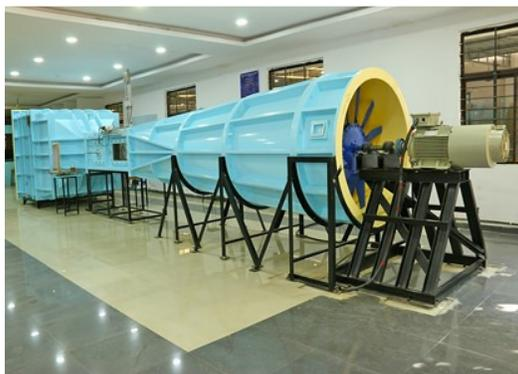
**Fig. 9.** Low-speed Wind Tunnel
