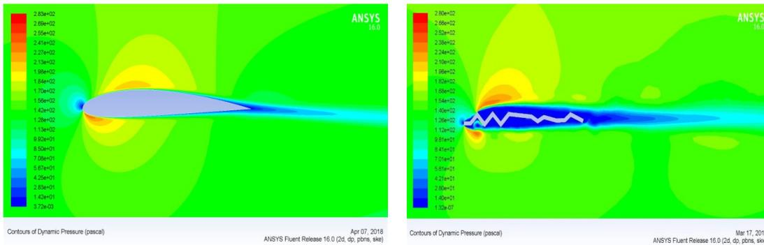
Fig. 26. Dynamic Pressure and Velocity Magnitude contours at AoA= 10 Deg, V= 15.4 m/s
