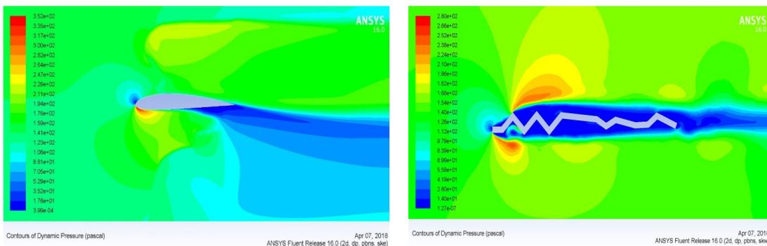
Fig. 27. Dynamic Pressure and Velocity Magnitude contours at AoA= 15 Deg, V= 15.4 m/s
