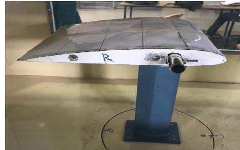
Fig. 15. Models Mounted on a six component strain gauge balance strut
