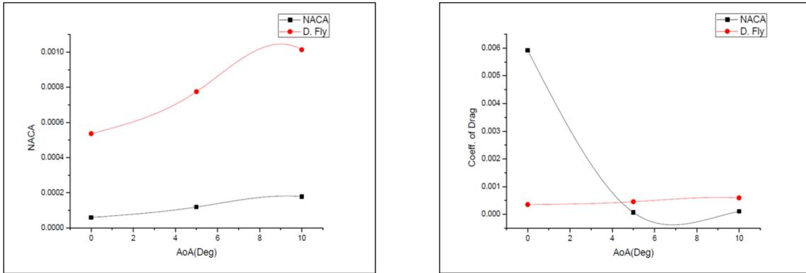
**Fig. 19.**  $C_d$  vs AoA plot for Experimental Results of airfoil at  $V = 11.8$  m/s and  $V = 15.4$  m/s
