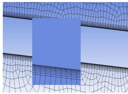
**Fig. 8.** Inflation layers over the surface of Dragonfly Airfoil
