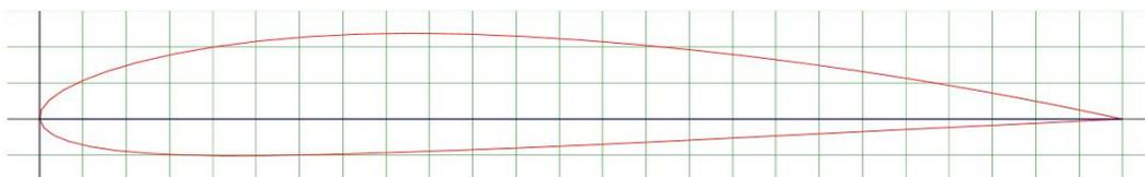
**Fig. 11.** Geometry of NACA 2.5411 Airfoil generated in Airfoil tools
