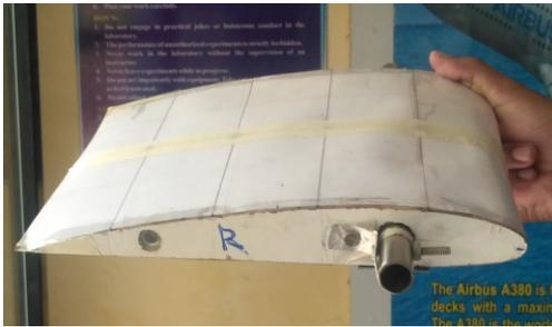
Fig. 13. NACA 2.5411 Airfoil Fabricated Model
