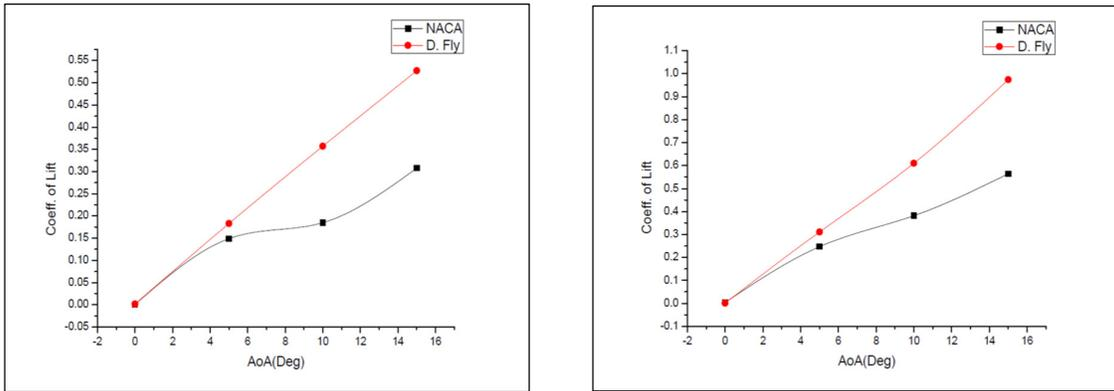
Fig. 16.  $C_l$  vs AoA plot for Numerical Results of airfoils at  $V= 11.8$  m/s and  $V=15.4$  m/s
