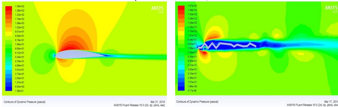
**Fig. 20.** Dynamic Pressure and Velocity Magnitude contours at AOA= 0 Deg,  $V = 11.8$  m/s
