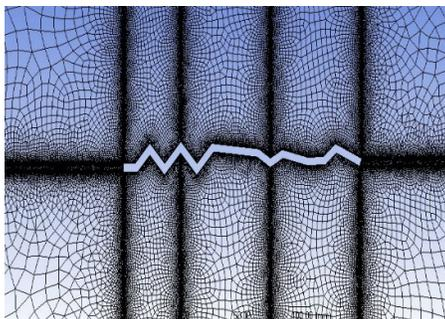
**Fig. 7.** Expanded view of the Dragonfly Airfoil's mesh
