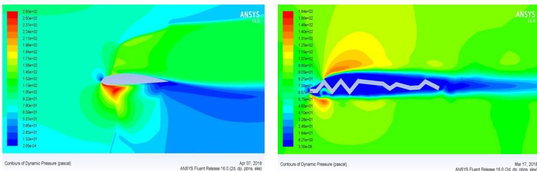
**Fig. 23.** Dynamic Pressure and Velocity Magnitude contours at AOA= 15 Deg, V= 11.8 m/s
