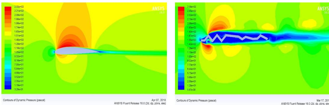
**Fig. 25.** Dynamic Pressure and Velocity Magnitude contours at AoA= 5 Deg, V= 15.4 m/s
