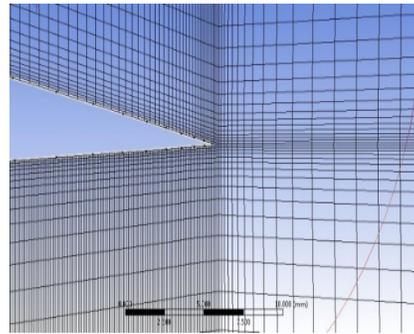
**Fig. 6.** Mesh at the trailing edge of NACA 2.5411 Airfoil
