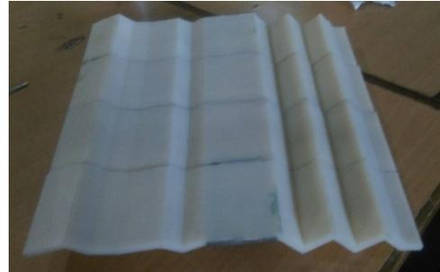
Fig. 14. Dragonfly Airfoil Fabricated Model
