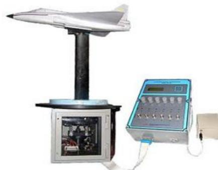
**Fig. 10.** Six Component Balance
