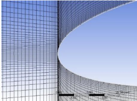
**Fig. 5.** Mesh at the leading edge of NACA 2.5411
