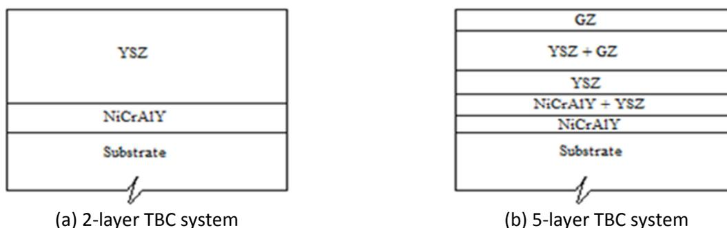
**Fig. 1.** Sketches of TBC systems used, where (a) for typical YSZ powder and (b) for GZ powder
