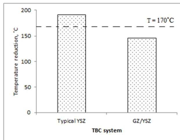
**Fig. 5.** Temperature reductions by both TBC systems at 1250°C
