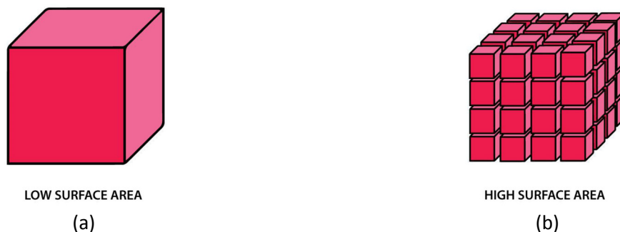
Fig. 2. Illustration image of comparison between (a) large particle with low surface area and (b) small particle with high surface area
