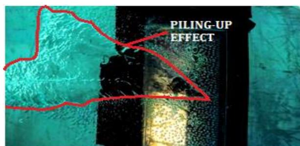
**Fig. 10.** Visual air bubbles that form on the vessel with the  $F_n$  0:13 and injection ratio 0.6
