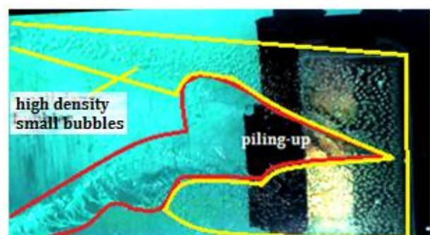
**Fig. 13.** Visual air bubbles that form on the vessel with the  $Fn$  0:29 and injection ratio 0.6
