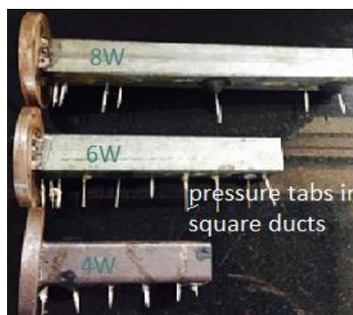
Fig. 5. Different L/W ratio ducts
