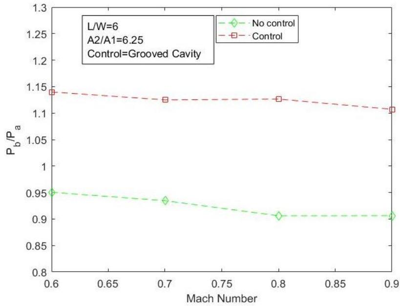
**Fig. 7.** Variation of Base Pressure against Mach number for L/W=6
