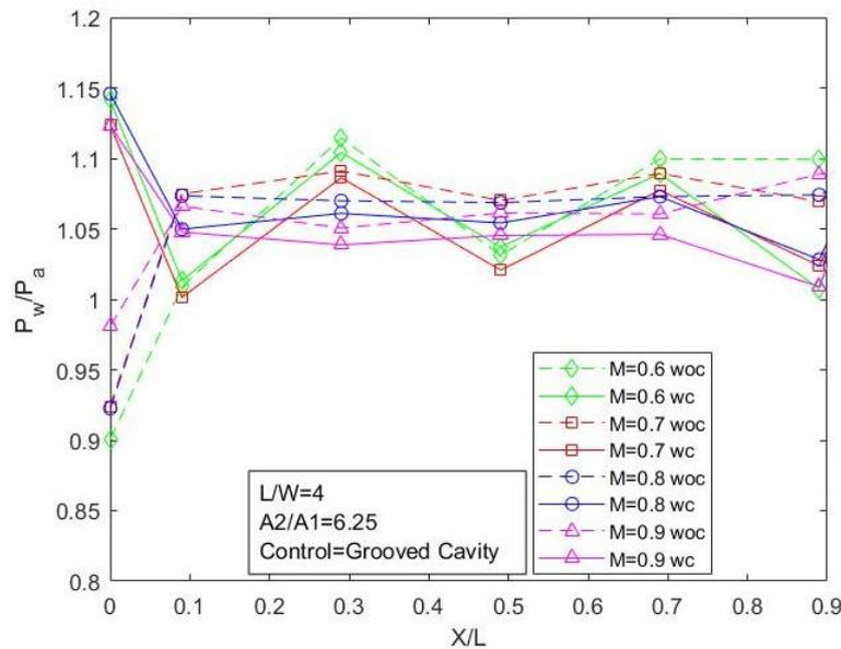
Fig. 11. Wall pressure distribution for  $L = 4W$
