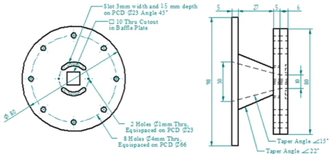
Fig. 4. Square nozzle and grooved control plate
