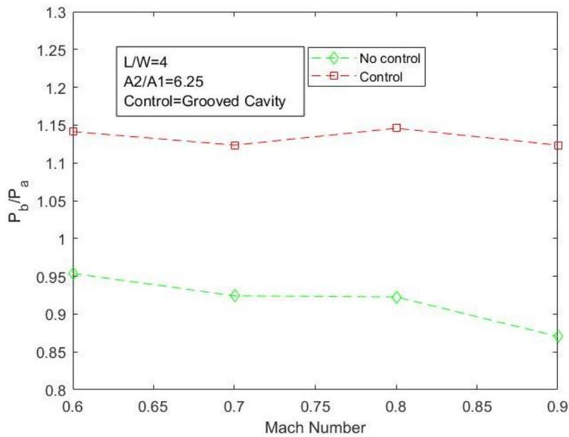
**Fig. 8.** Variation of Base Pressure against Mach number for L/W=4
