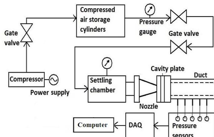
Fig. 3. Schematic description of experimental Setup
