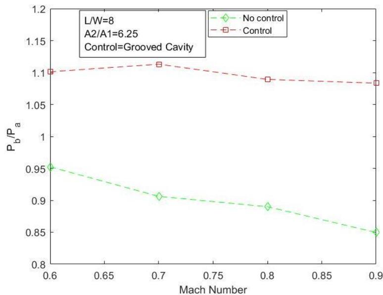
**Fig. 6.** Variation of Base Pressure against Mach number for L/W = 8
