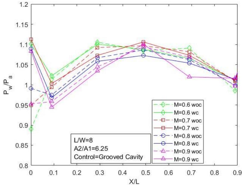
**Fig. 9.** Wall pressure distribution for  $L=8W$
