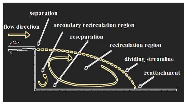
Fig. 1. Mixed flow field behind Backward Facing Step
