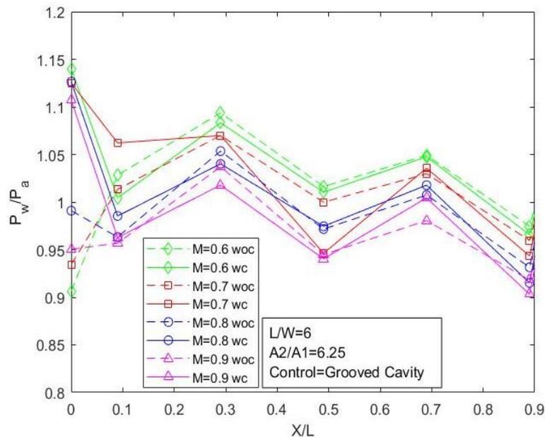
**Fig. 10.** Wall pressure distribution for  $L = 6W$
