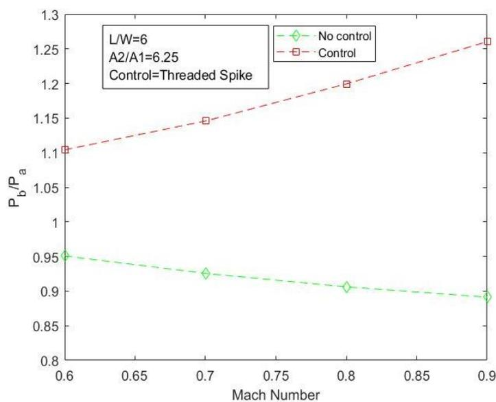
**Fig. 9.** Variation of Base Pressure against Mach number for  $L/W = 6$
