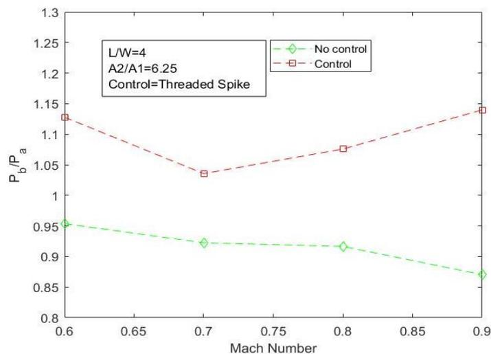
Fig. 8. Variation of Base Pressure against Mach number for L/W = 4
