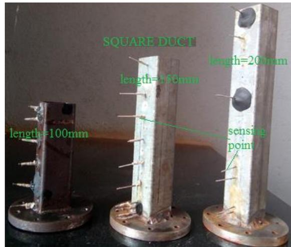
Fig. 7. Different L/W ratio ducts
