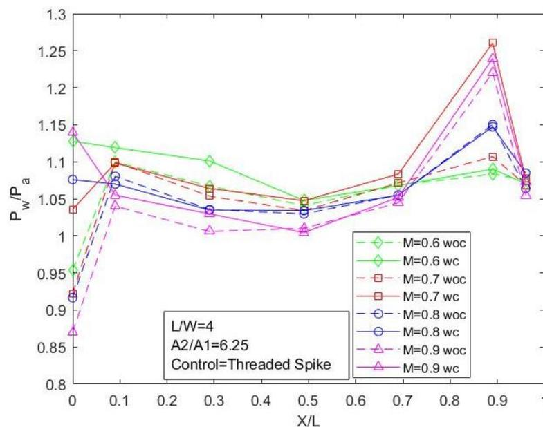
**Fig. 11.** Wall pressure variation at different regimes for  $L=4W$
