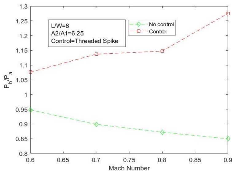
**Fig. 10.** Variation of Base Pressure against Mach number for  $L/W = 8$
