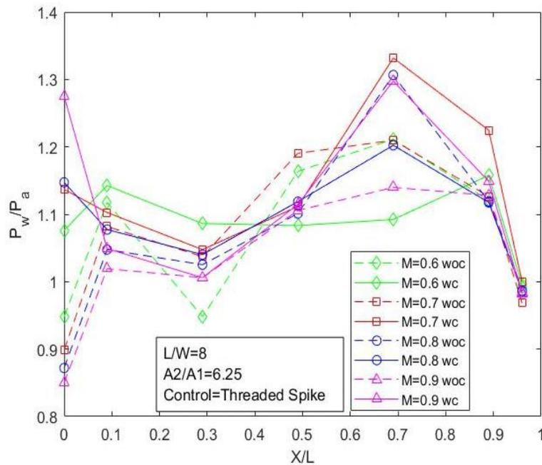
**Fig. 13.** Wall pressure variation at different regimes for  $L = 8W$
