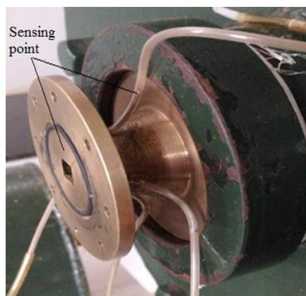
**Fig. 6.** Control plate with spike plate
