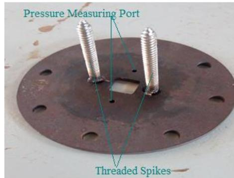
**Fig. 5.** Control plate with threaded spike
