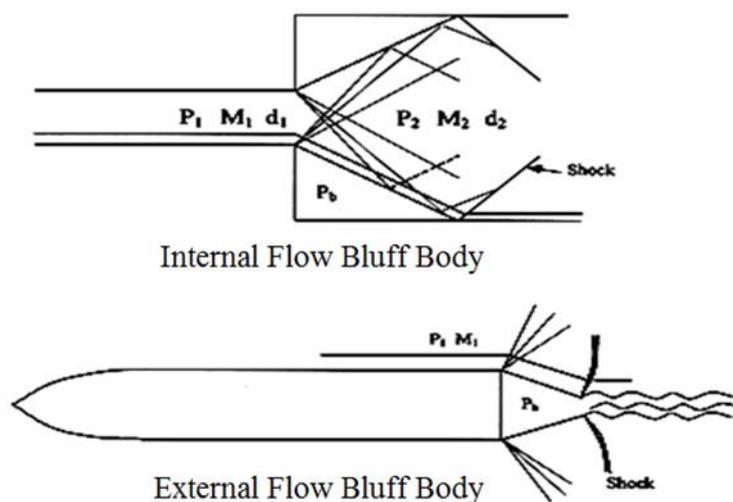
Fig. 1. Internal and External Flow Bluff Body
