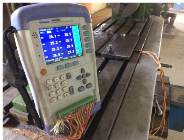
Fig. 5. The data logger used in measuring temperature
