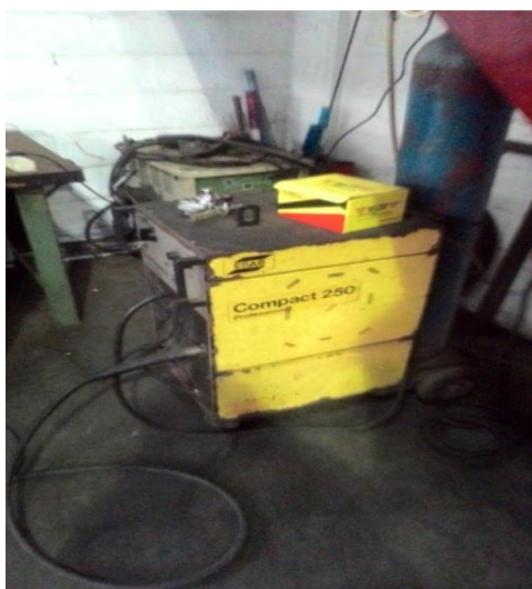
Fig. 1. The ESAB Compact 250 GMAW machine
