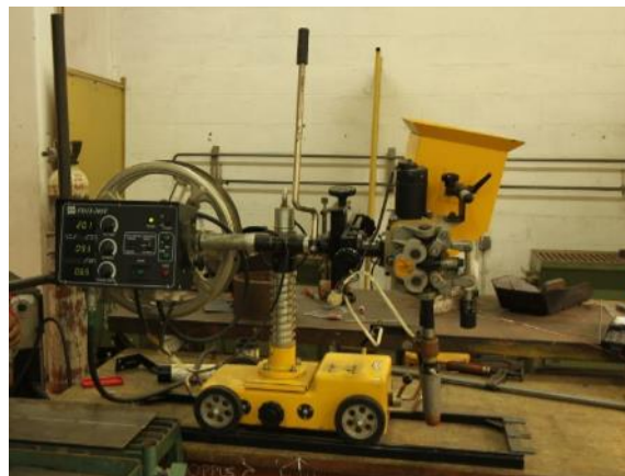
Fig. 2. The mechanism to control welding speed
