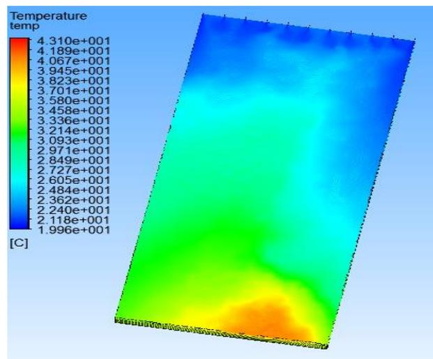
**Fig. 11.** Temperature distribution of PV panel at inlet water temperature of 20 °C
