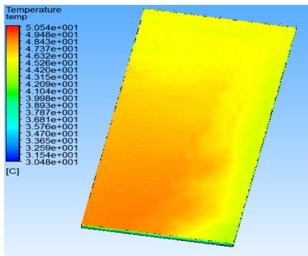
**Fig. 16.** Temperature distribution of PV panel at inlet water temperature of 45 °C
