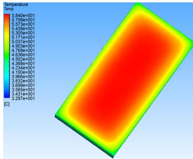
**Fig. 9.** Temperature distribution of PV panel without cooling system
