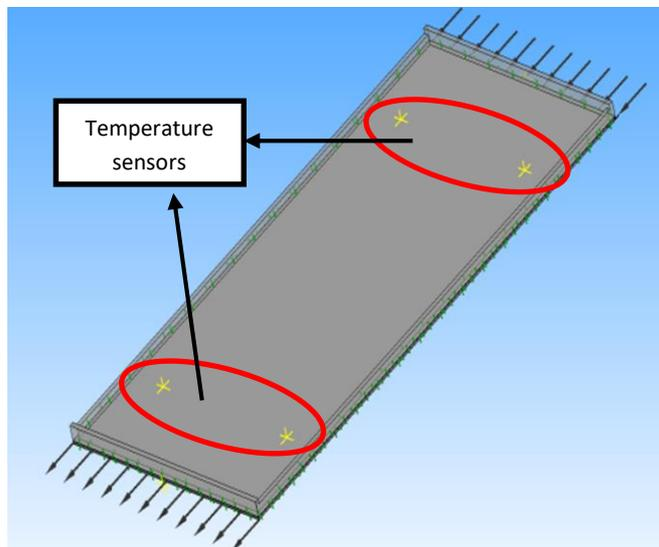
**Fig. 4.** Temperature sensors placed at backside of geometry model
