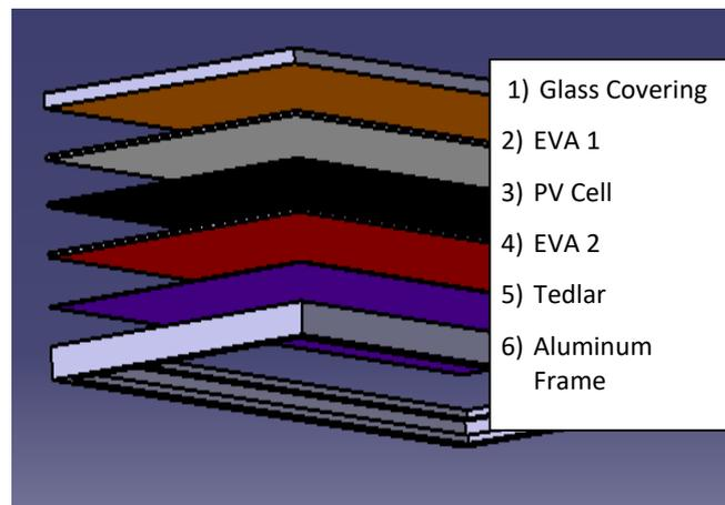
**Fig. 1.** Sketch of the geometry model of PV panel without cooling system
