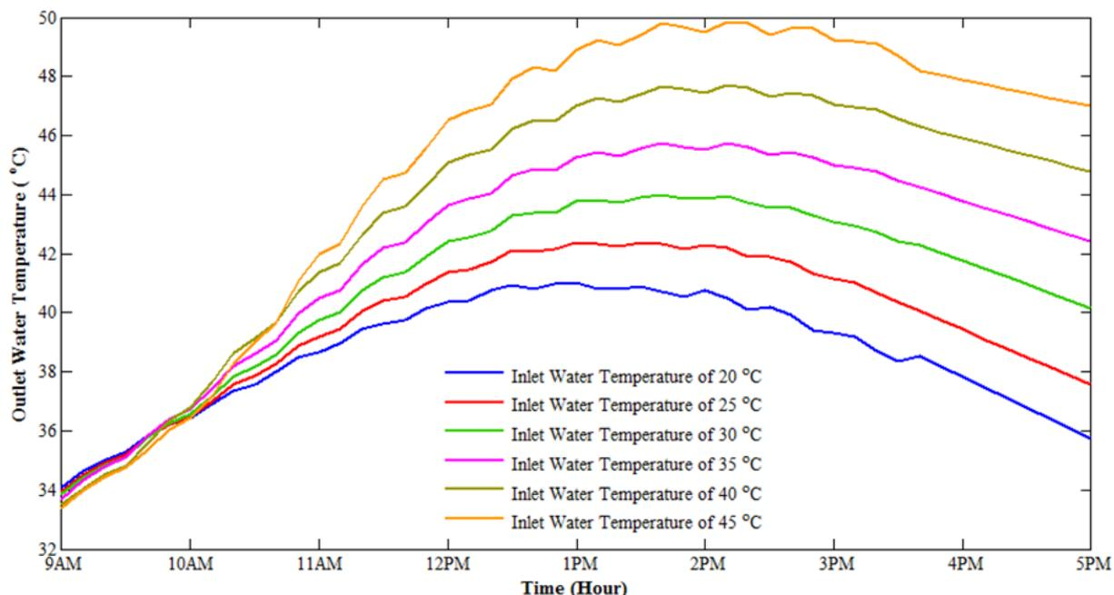
**Fig. 17.** Temperature of outlet water flow for each of the PV panel with water cooling system
