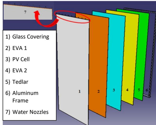
**Fig. 2.** Sketch of the geometry model of PV panel with water cooling system
