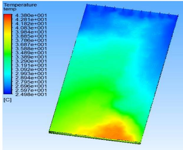
**Fig. 12.** Temperature distribution of PV panel at inlet water temperature of 25 °C
