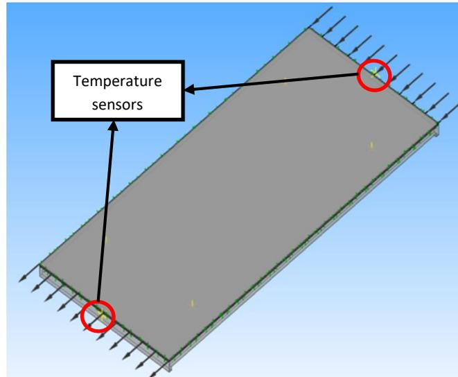
**Fig. 5.** Temperature sensors installed at inlet and outlet of water cooling
