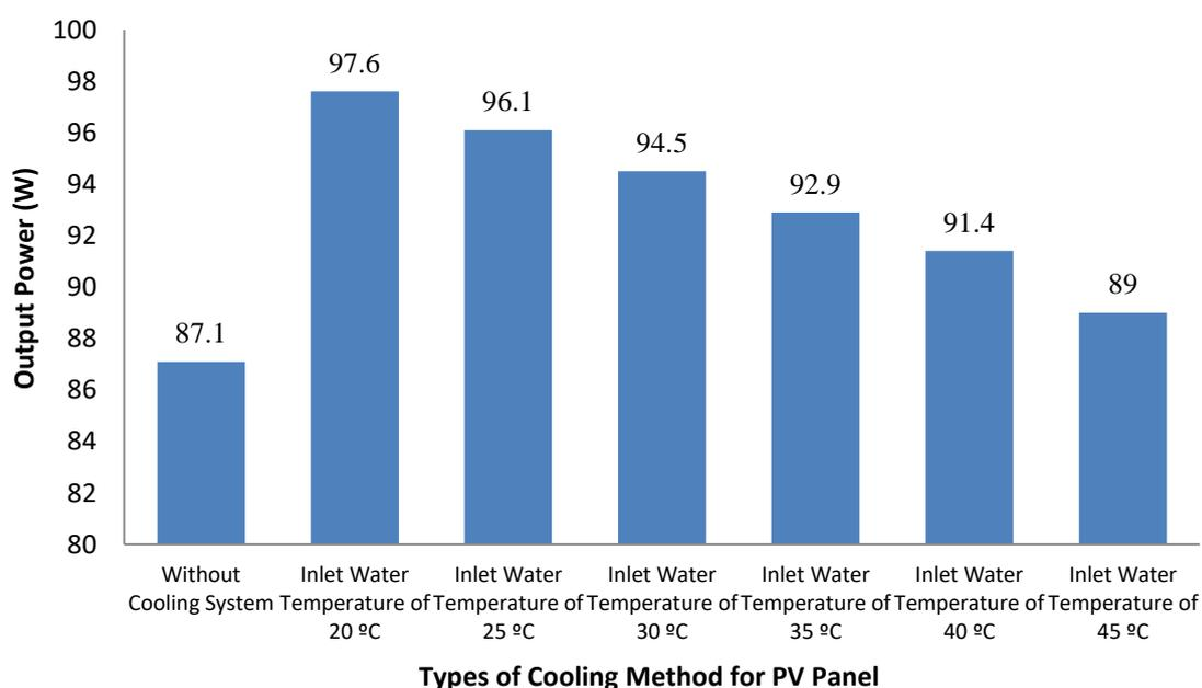
**Fig. 18.** Output power generated by the PV panels without and with water cooling system
