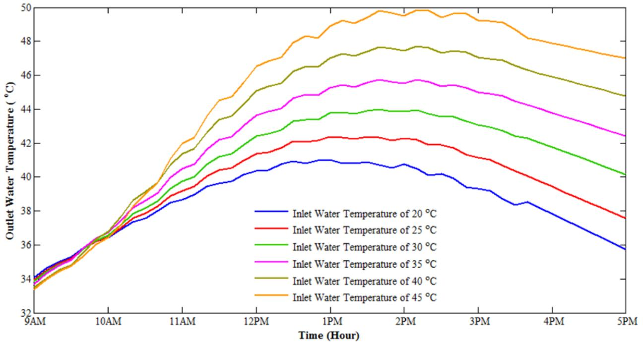
**Fig. 10.** Temperature of PV panel under different inlet water temperature
