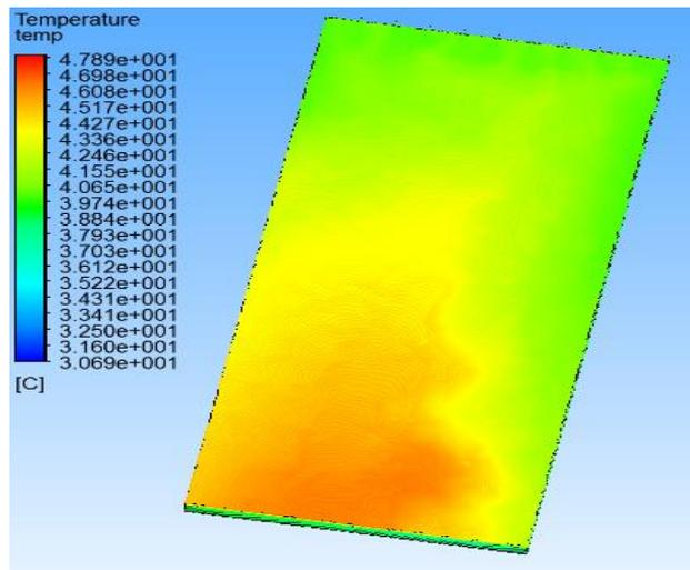
**Fig. 15.** Temperature distribution of PV panel at inlet water temperature of 40 °C
