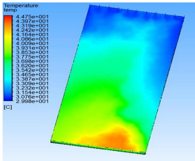
**Fig. 13.** Temperature distribution of PV panel at inlet water temperature of 30 °C
