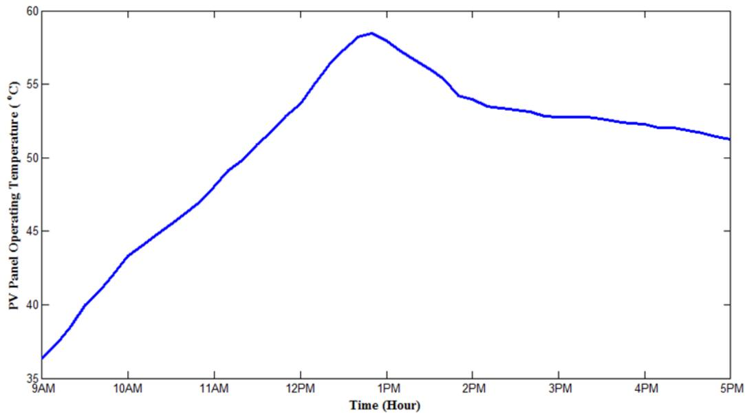
**Fig. 8.** Temperature of PV panel without cooling system
