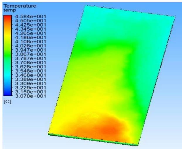
**Fig. 14.** Temperature distribution of PV panel at inlet water temperature of 35 °C
