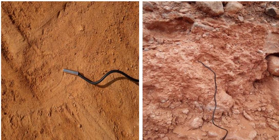
**Fig. 3.** Temperature sensor with 10 cm inside soil layer
