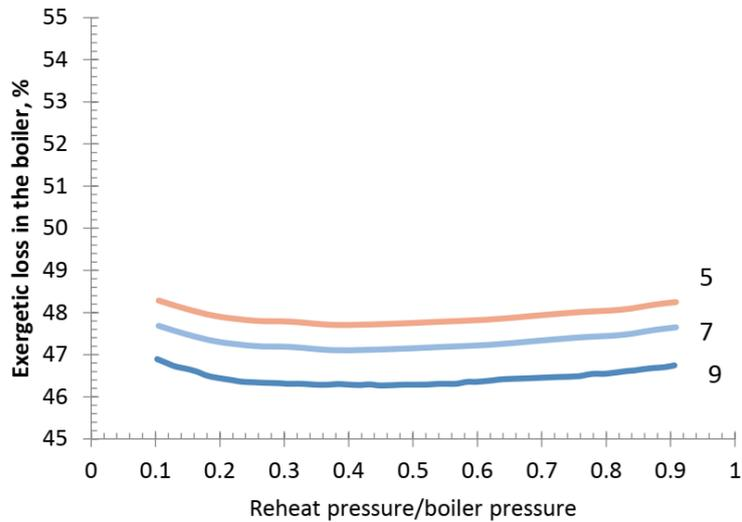
**Fig. 3.** Effect of number of FWHs with reheat pressure on exergetic loss in boiler
