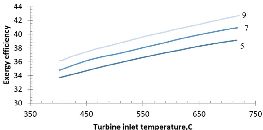
**Fig. 5.** Effect of turbine inlet temperatures with number of FWHs on the exergy efficiency.
