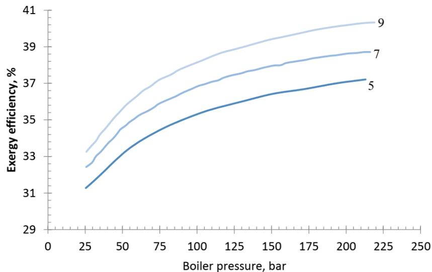
**Fig. 4.** Effect of boiler pressures with number of FWHs on exergy efficiency
