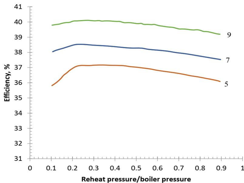
**Fig. 2.** Effect of number of FWHs with reheat pressure on exergy efficiency
