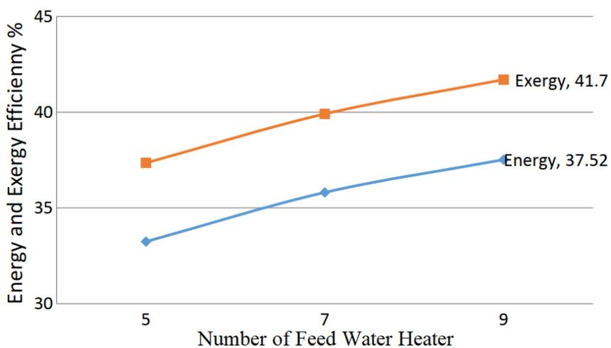
**Fig. 6.** Thermal Efficiency of the Cycle
