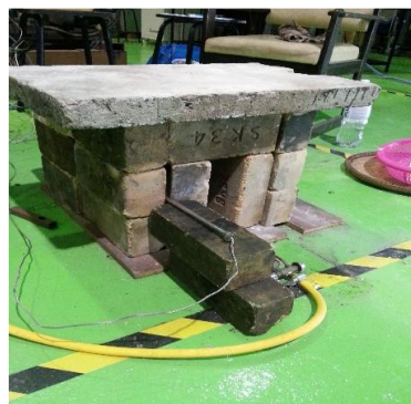
Fig. 4. Thermocouples at the interior wall
