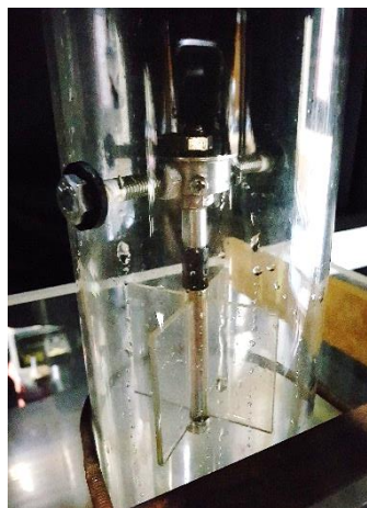
Fig. 2. Swirl meter in compliance with ANSI-HI 9.8 (2012) [14]
