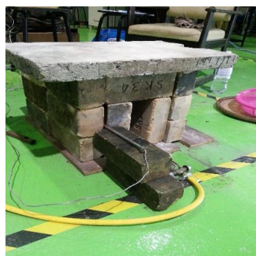
Fig. 4. Thermocouples at the interior wall
